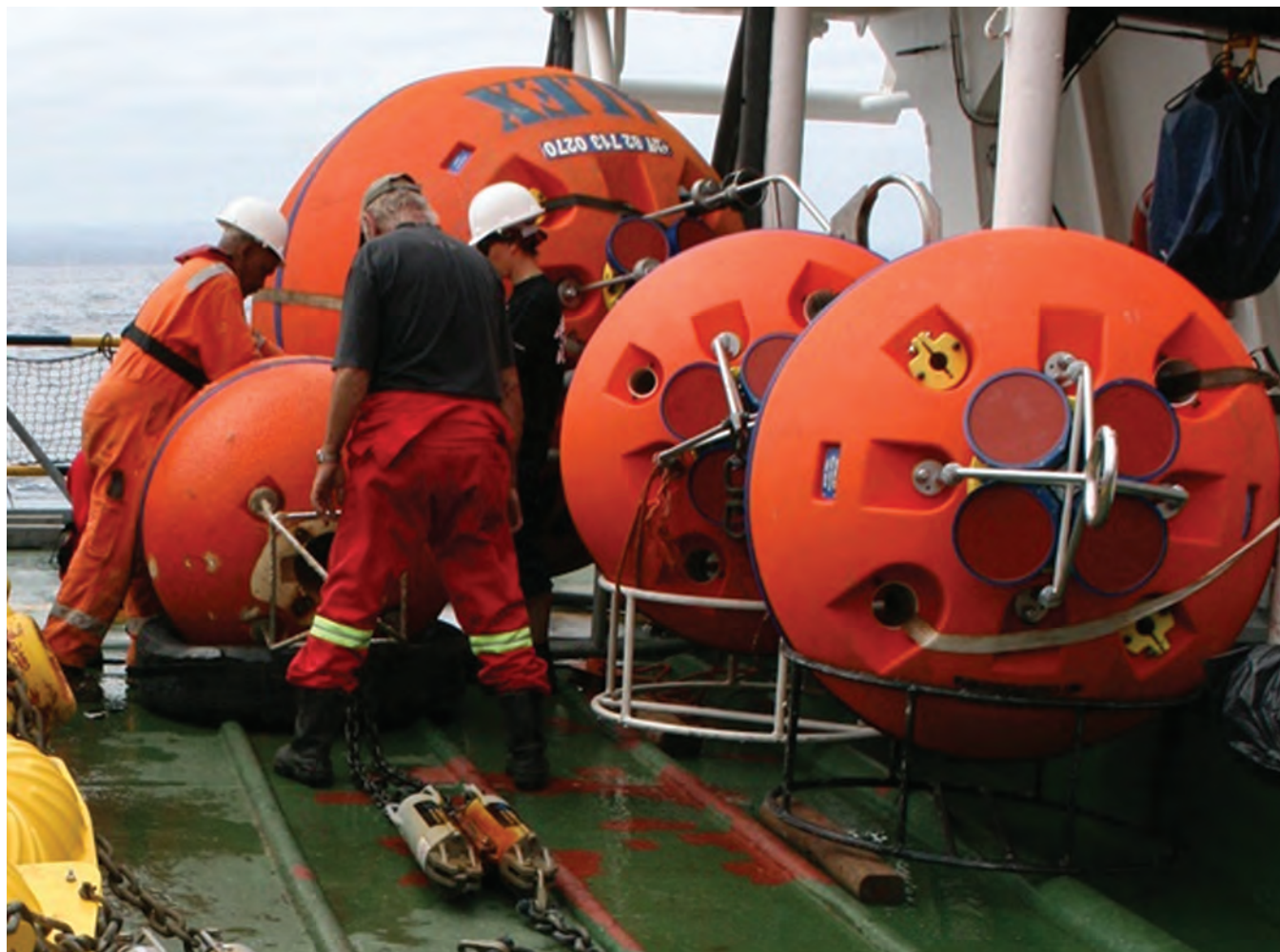
Teledyne RDI ADCPs seated in Top Buoys of ASCA Mooring Array.
