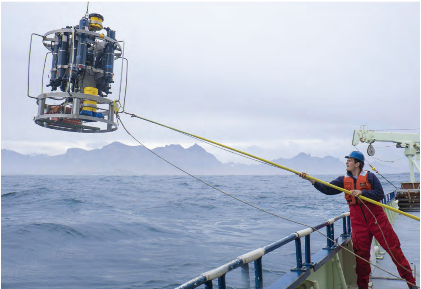
Fig. 6: Hydrographic package with dual Teledyne RDI ADCPs (yellow) in action off Greenland.
