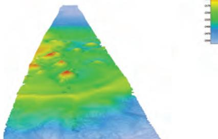
**Color coded bathymetry of multibeam data contributed by Fugro from a recent transit that shows seamounts on the surrounding seafloor.**
