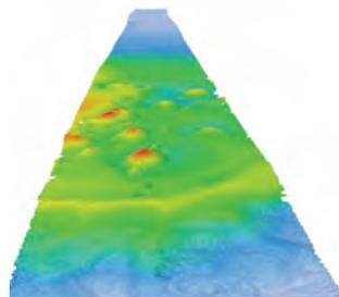
**Color coded bathymetry of multibeam data contributed by Fugro from a recent transit that shows seamounts on the surrounding seafloor.**
