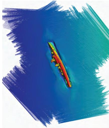
**Color coded bathymetry showing sunken vessel on seafloor.**
