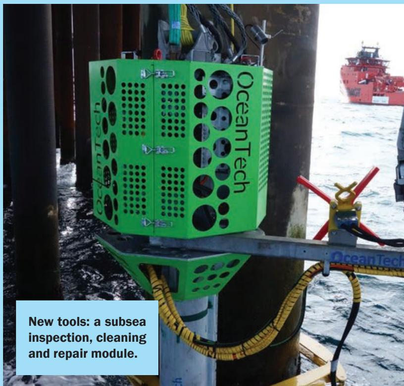
**New tools: a subsea inspection, cleaning and repair module.**
