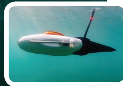
Nicknamed Poggy, the AUV is a one of a kind, novel bionic design with two propulsion thrusters and two independent flexible “tails” that give the robot unique mobility features.
