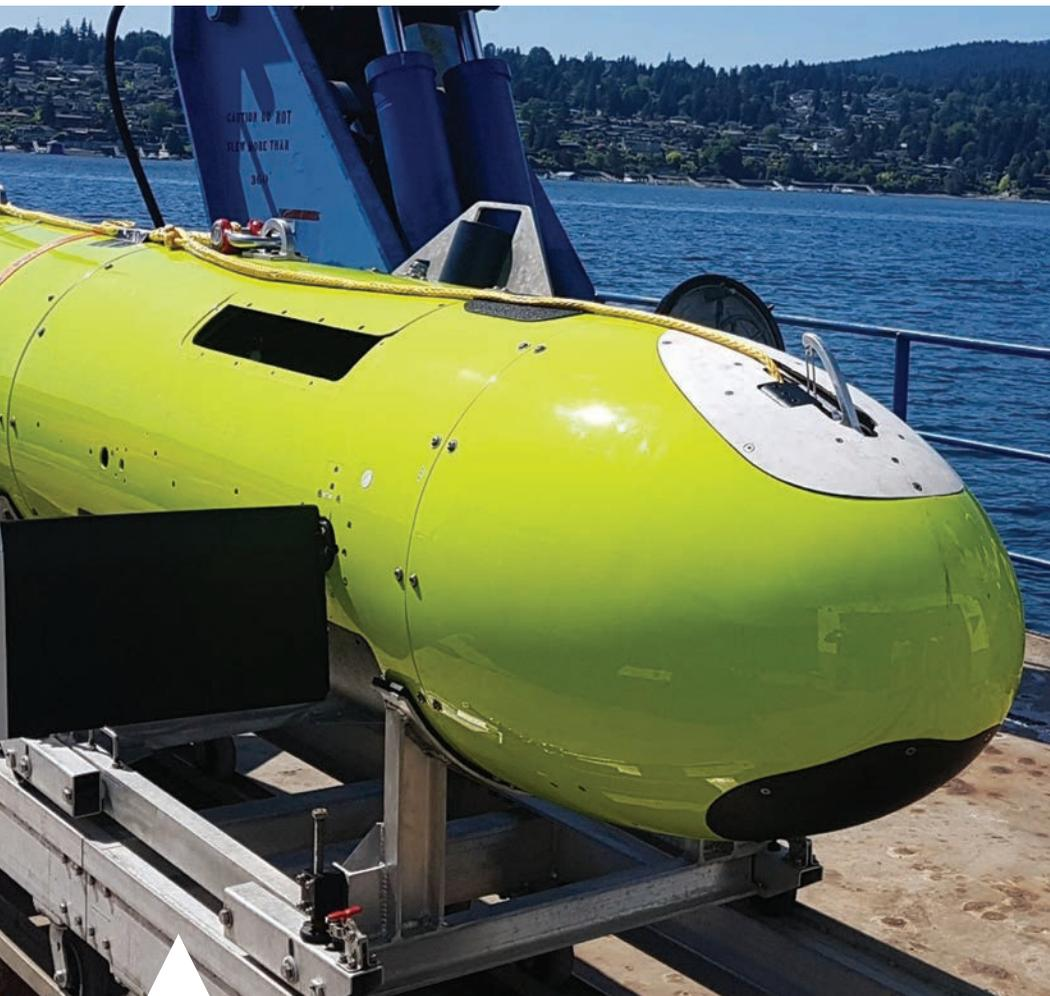
AUV fit with nose hook capture mechanism connected directly to dorsal lift lugs.
