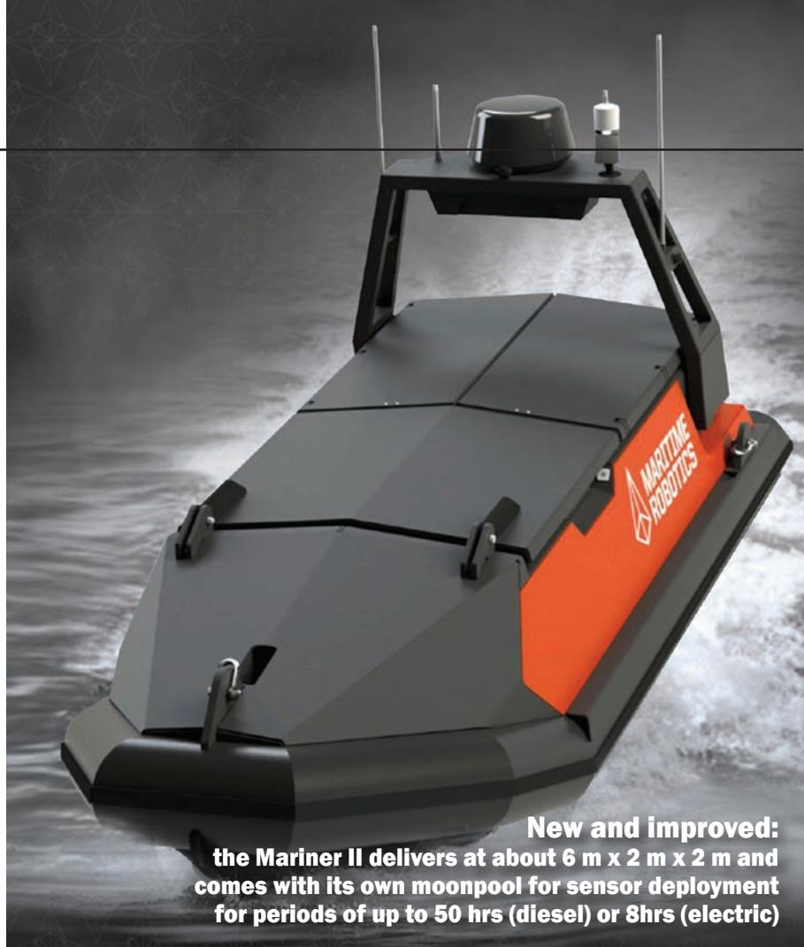
**New and improved: the Mariner II delivers at about 6 m x 2 m x 2 m and comes with its own moonpool for sensor deployment for periods of up to 50 hrs (diesel) or 8hrs (electric)**
