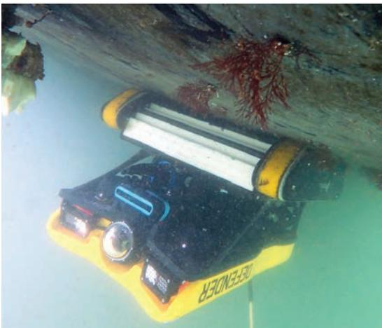
New Greensea crawler technology shown with the VideoRay ROV supports UWILD and EOD hull inspections.
