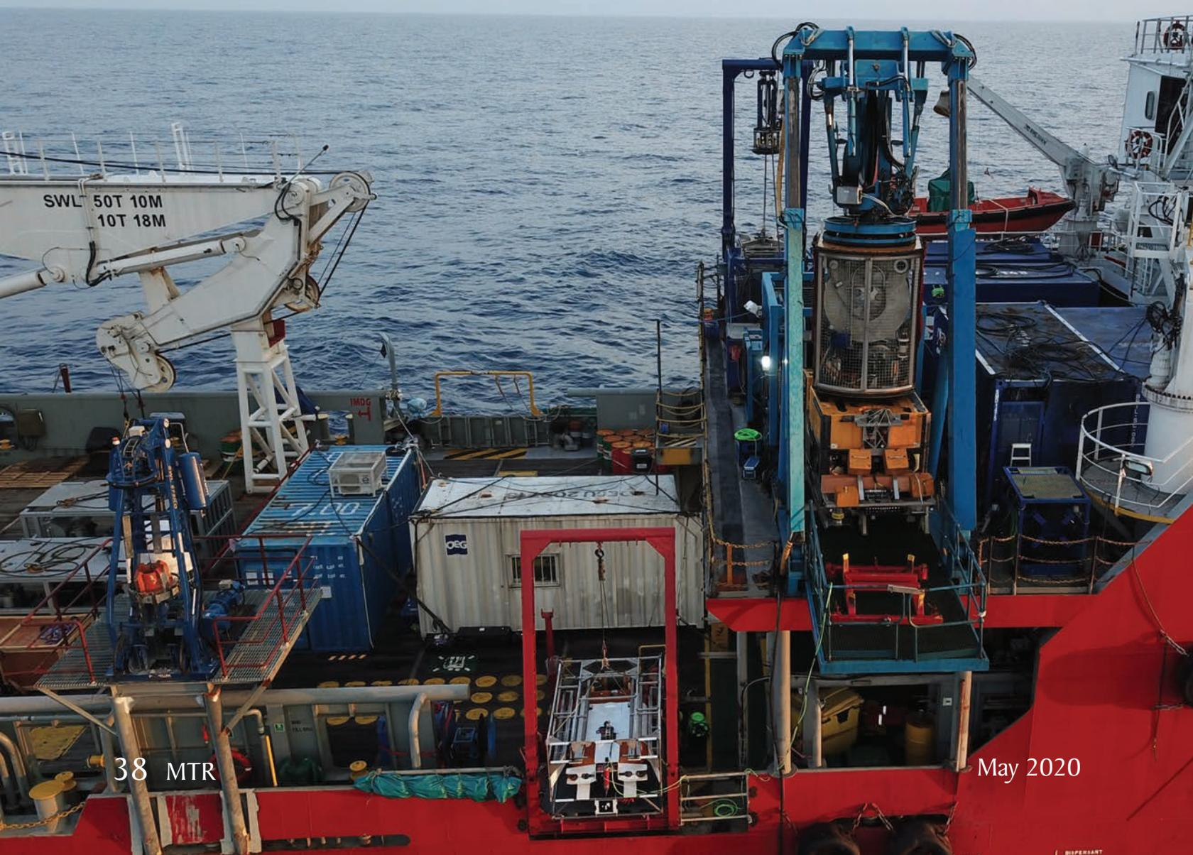
autonomous exit and re-entry of its cage, auto search for pipeline targets, auto-pipe tracking and semi-autonomous approach to a riser flange on a well head platform. During these trials, the AUV was fitted with an AvTrak 6 tracking and telemetry beacon, was tracked using a rented Mini-Ranger 2 USBL and used WSM 6+s on the cage for homing.
