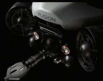
FUSION is an expeditionary hybrid AUV/ROV with a bespoke suite of high-end sensors delivering a highly capable and intelligent system. A self-contained (no generator required) system augmented by clever automation and supervisory control through an unparalleled, intuitive user interface establishes a new benchmark in UUVs.
