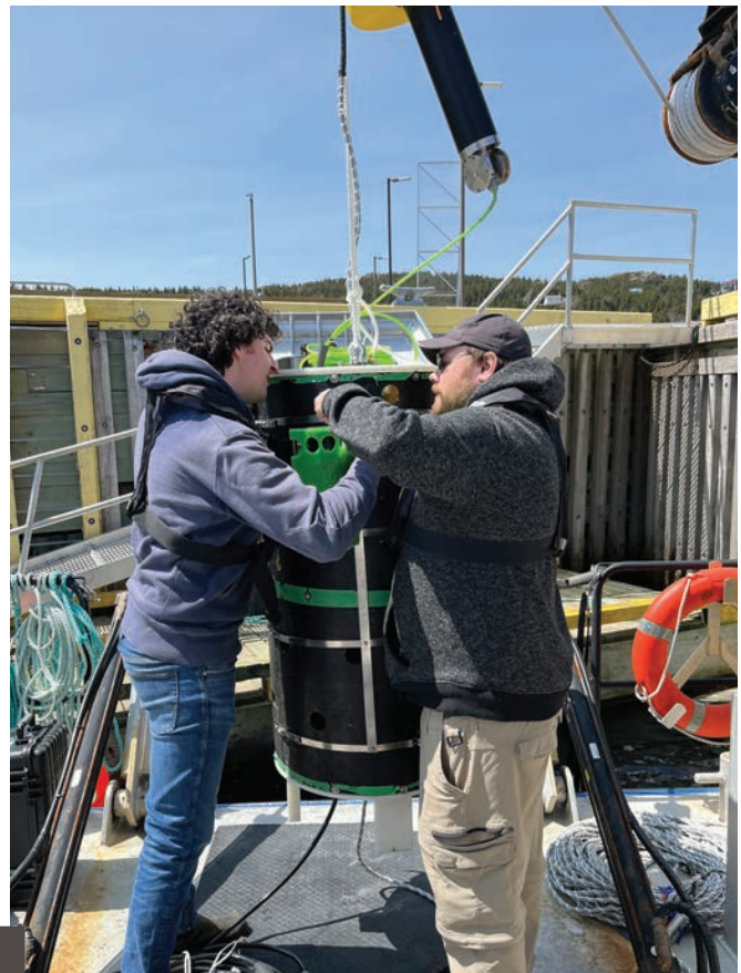
eSonar staff Matt Dinn and Cory Parsons preparing a hydrophone array mooring prior to deployment onboard the RV Lucy Pudluk at “The Launch” facility of Marine Institute (Memorial University).
