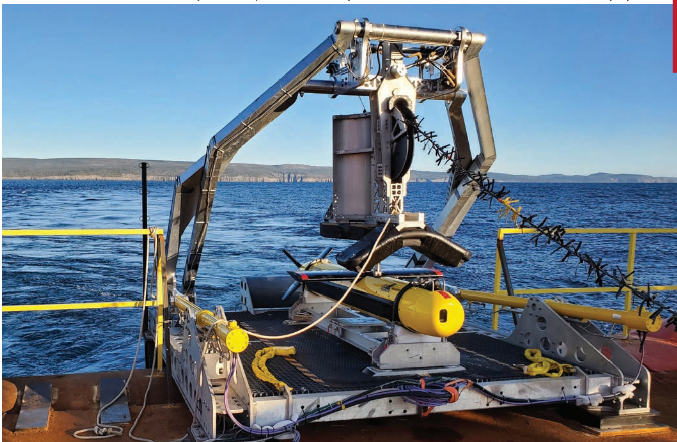
Kraken KATFISH towed synthetic aperture sonar system and autonomous launch and recovery system.
