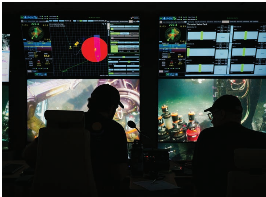
Silhouetted against screens, Remotely Operated Vehicle pilots take vibracorer samples using ROV SuBastian.
