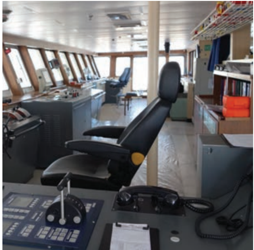
Bridge deck modified to comply with ECDIS and DP2 station keeping.
