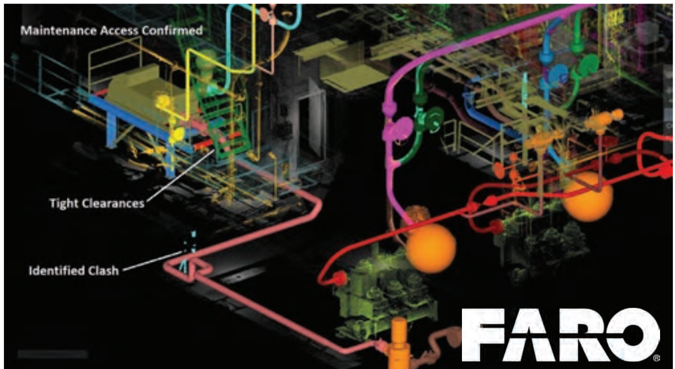
New Equipment installed in 3D Point Cloud model. Note: a clash was resolved during installation and the tight clearances necessitated that the pump was shoehorned in under the stairway.
