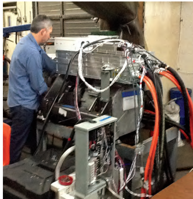
BAE Hybrid Drive traction motor during Factory tests in Seattle.
