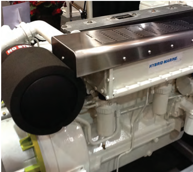
Northern Lights & Luger Engine generator engine coupled to BAE Hybrid Drive
