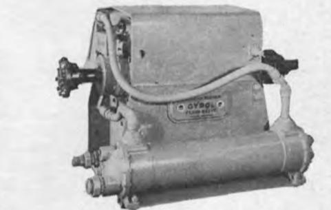
GYROL FLUID DRIVE Type VS—class 2—Dual rotation. Mfg by American Blower—complete with oil cooler. Speed range 200 R.P.M. minimum to 1750 R.P.M. maximum. Unit locates between motor and pump. Suitable for pumping molasses, oil products, etc.
