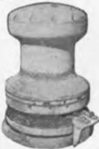
Hesse-Ersted Vertical, Single Wildcat—for 1 3/8" Anchor Chain, single gypsy, with 35 HP General Electric Motor, 230 Volts DC, complete with Controller equipment.
