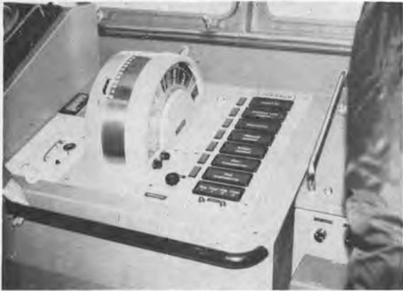
Simplified bridge console of the FAHM type gives the deck officer full control of the main propulsion plant.
