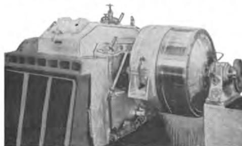
1-port, 1-starboard, ratio 2.292:1, rated 2000 HP, with Fawick Clutches.
