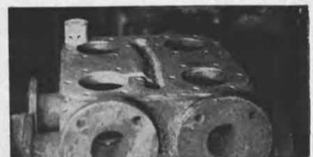
This cracked water manifold was prepared for welding BUT—due to the pressure of time the vee'd cracks were filled with Cordobond Strong-Back Steel Putty (in lieu of welding). Repair time 4 hours including curing, and testing to 3 times the working pressure.
