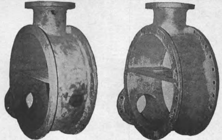
This auxiliary condenser water box offers just one more example of the excellent results obtained with the Cordobond Strong-Back Method. Holed through area was repaired by Cordobond Strong-Back method using Cordobond Strong-Back putty.
