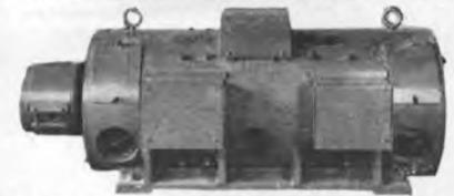
BURKE: Unused—5KW—Input 9.4 HP/120 volts DC/1800 RPM/71 amps. Output 5 KW 10 KVA—120VAC/1/60—52 amps—0.5 PF. With Ward Leonard speed controller.
