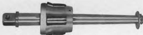
Expanders for tubes up to 4 1/2" OD roll and flare in one operation. Models for parallel or non-parallel expanding.
