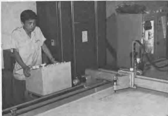
Technician at Nippon Kokan monitors operation of computer-controlled equipment automatically preparing hull form line drawings for ship designs and cost estimates.
