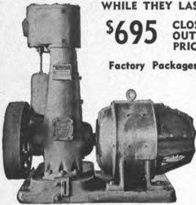
120 volts DC—400 RPM—drip-proof marine type. 2-Wire direct connected set. Reciprocating 6 x 7 type E vertical self-oiling steam engine—plug & piston valve—220 lbs PSI—80 lbs. BP.
