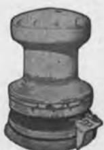
3—Hesse-Ersted Vertical, Single Wildcat—for 1¾" Anchor Chain, single gypsy, with HP General Electric Motor, 230 Volts DC, complete with Controller equipment.
