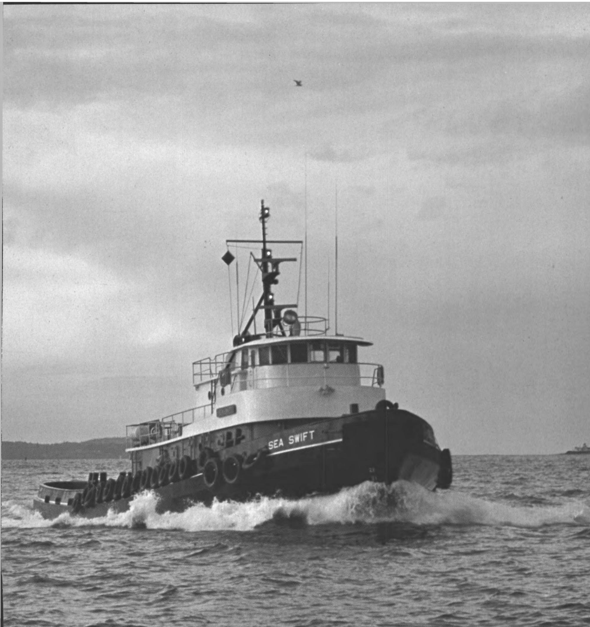
The twin-screw Red-Stack tug, Sea Swift is powered by two General Motors 16-645E5 Diesel engines which are controlled from the pilot house by GM pneumatic control equipment. In calmer seas, she can cruise at 15 knots under tow.
