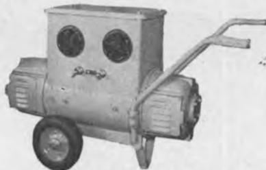
Motor: 10 HP—230 volts DC—2800 RPM. 200 amps max. continuous welding. Range regulation 15/200 amps. Dimensions: 38" X 30" X 20". Weight: 514 lbs. Shipping case—48" X 35" X 25". Complete with 100 ft. welding cable—ground clamp & electrode holder. Built to Lloyd's—Register BS 638—1954.
