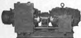
Janette M-G Sets. Input: 1.75 HP, 230 V, DC, 7.2 Amperes, 1800 RPM. Output: 1-KVA (.85 KW), 115/1/60, 4 ball bearing, with speed regulator, and with noise filters. Navy Type CJM-21151, continuous duty. Net weight 435 #, Dimensions 44" L, 19½" W, 18½" H. Instruction book and parts list included.
