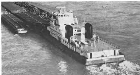
**Lillian Clark.** Her twin new-series EMD diesels are each rated 3,225 continuous bhp at 800 rpm. Engines have been lubricated with Shell TORNUS Oil since launching.
