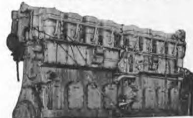
Type LS — 15 1/2 x 22 — turbo-charged engine—BHP 1300 @ 270 RPM. Air starting @ 250 lbs. Complete with air tanks, heat exchanger and all accessories. Preserved in equal-to-new condition. Also spare pistons, cylinder liners, valves, etc. Still aboard Corps of Engineers vessel. Serial No. 2172 —Buchi Turbo-charged.
