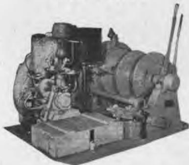
Small general purpose winches, mfg by Jaeger. Rated 2500 lbs @ 75 FPM. Driven by air-cooled Enfield single Cylinder diesel engine. Decutchable free spooling drum has center flange which can be removed if required. Excellent for small vessel use and general purpose service on all vessels. Has spare parts box. Weight about 1500 lbs.
