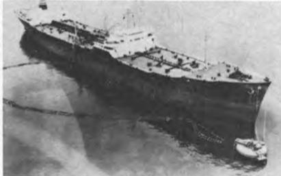
rotate about the SPM terminal with the tanker, connect the ship's cargo manifolds to the SPM. Other hoses connect the underside of the SPM to the submarine pipelines.
