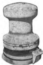
3—Hesse-Ersted Vertical, Single Wildcat—for 1 3/8" Anchor Chain, single gypsy, with HP General Electric Motor, 230 Volts DC, complete with Controller equipment.
