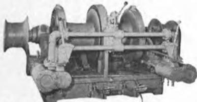
Drum 8500 lbs @ not less than 120 FPM; 13,000 lbs at no specified speed. Gypsy head 22,500 lbs. static pull. Foot brake to hold 17,000 lb. pull. Steam cylinders with standard 250 PSI. DIMENSIONS:
