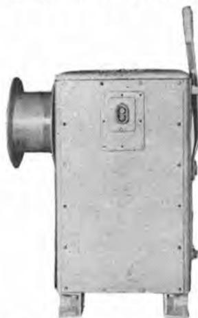
Designed for use with Bathythermograph—Submarine Signal Co.—type E/2/S—without cables—single speed 300 lb. pull @ 360 FPM—single drum 9" X 6 3/4"—with 1 7/8" flanges—clutch controlled with pawl & ratchet. Designed for use with 1200 ft. of 1/8" stainless cable. Motor: 3 HP—440/3/60—1700 RPM—intermittent. 5 Available—Navy surplus—show little use.
