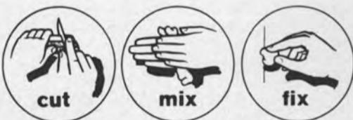
EPOXYBOND is unmatched in its versatility. It mixes like putty and hardens like steel. It adheres to metal, wood, and other materials—even when surfaces are damp—and it sets under water!
