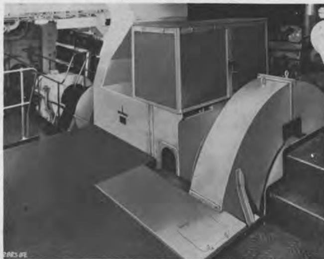
Figure 2—Synchronous generator fitted in line of shafting.
