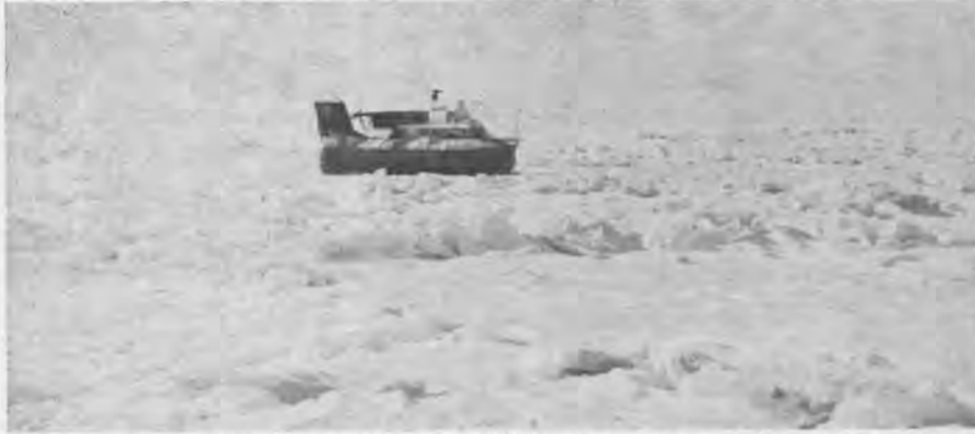
Riding on its four-foot cushion of air, the ACV is shown out on Lake Erie ice where it attained an average speed of 30 miles per hour while covering 2,700 square miles.
