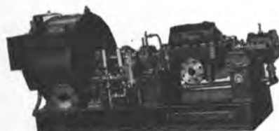
MAIN FEED PUMP
