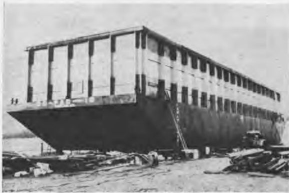
DELIVERED BY SCHNITZER: Barge COPAC No. 10, shown on the ways at the Schnitzer yard in Portland, Ore., was recently delivered to Columbia Pacific Towing of Stevenson, Wash., by Schnitzer Leasing, division of Schnitzer Industries. The 150-foot by 45-foot by 12-foot barge with chip bin will be operated on the Columbia and Willamette Rivers servicing the expanded COPAC fleet.
