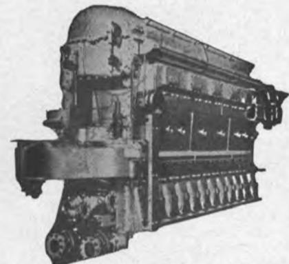
(4)—10 Cylinder—2-cycle—1800 HP @ 800 RPM. 8½x10—air starting—reversible. Complete with Harrison coolers, syphon valves, strainers, filters, etc. For immediate delivery.
