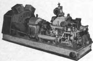
WESTINGHOUSE Turbines, 440 PSI, 740° F, with Westinghouse Generators, 250 KW, 120/240 DC.
