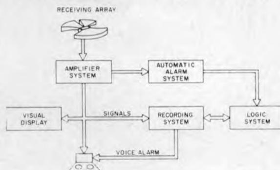
Figure 2—Block diagram of H-LAD system as currently being tested on the Edward B. Greene on the Great Lakes.
