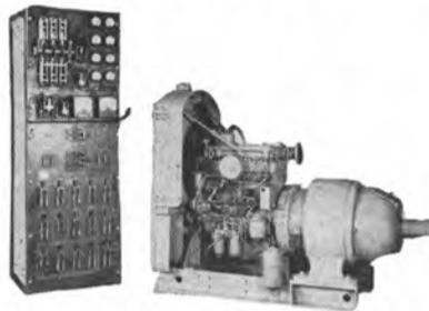
Hercules DOCC 4" X 4 1/2" diesel engine. Generator: Fidelity Electric—LCD3—15 KW—120/240 Volts DC—62.5 amps. With switchboard and automatic transfer switch. From C2-S-AJ2—North Carolina built. Good operating condition.
