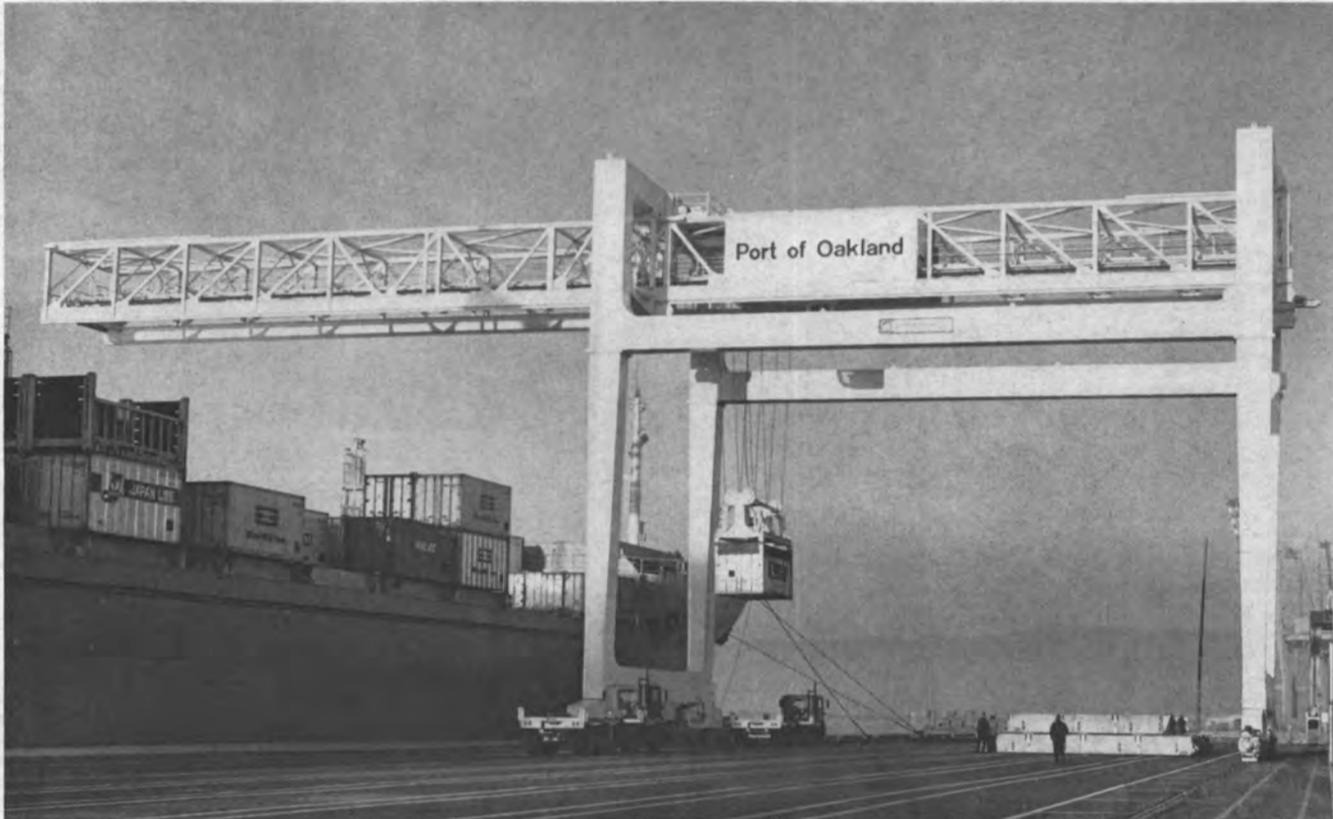
Built by PACECO for the Port of Oakland, this Low Profile Portainer not only loads and unloads container ships but also services the storage
