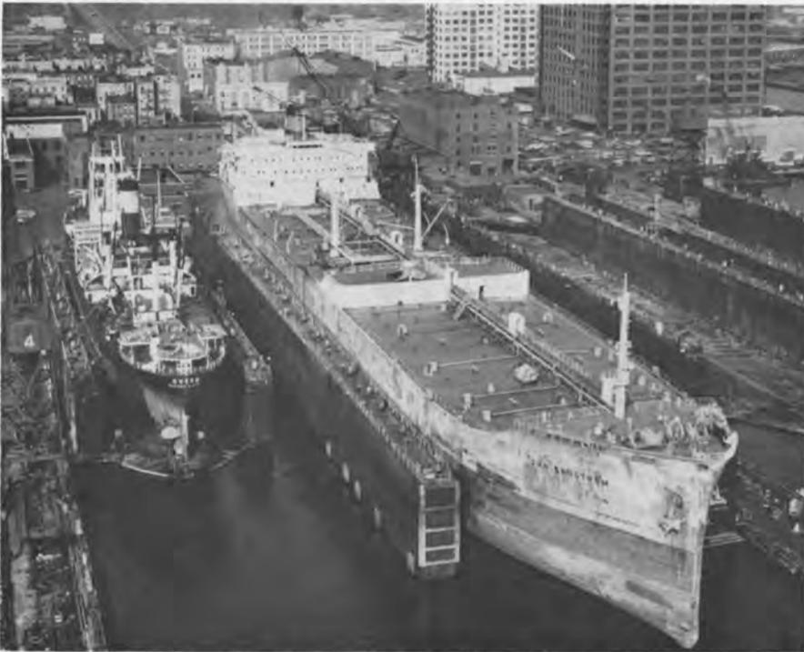
The largest tanker ever drydocked in the Port of New York, the 57,700-dwt Swedish motor vessel Dan Brostrom, sits high and dry at Bethlehem Steel's Hoboken, N.J., ship repair yard. Docked stern inboard, she overhangs outboard end of the dock about 100 feet. The tanker has an overall length of 773 feet 11 inches.
