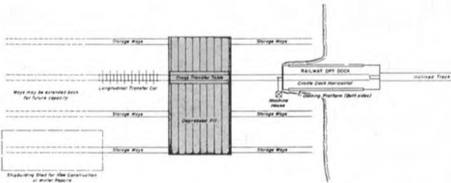
BASIC LONGITUDINAL TRANSFER SYSTEM FROM END HAUL RAILWAY OR FLOATING DOCK
