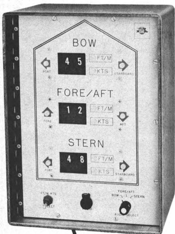
**A precision docking sonar system which utilizes the Doppler principle to provide absolute "over-the-bottom" velocity information for berthing of super vessels.**
