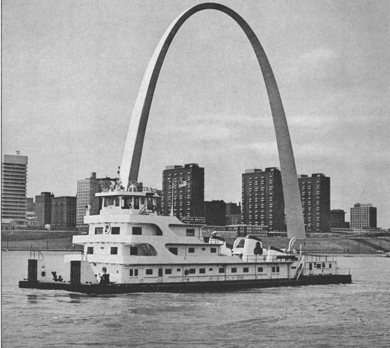
Rose Barge Line's elegant new 5000 h.p. M/V American Beauty is all the name implies. It incorporates the latest advancements of the **HYDRODYNE** Hull form with Kort nozzles, as recently tested at the Netherlands Ship Model Basin. No
