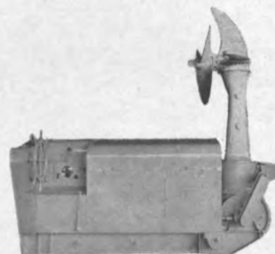
Model 02-D—powered by 6-cylinder G.M. 6-71 diesel—driven through Oliver gear—8708—forward ratio 1:1.27—reverse 1:1—3 blade propeller—48" diameter—24" pitch—left hand—manual steering—electric starting. RECONDITIONED—READY TO GO!
