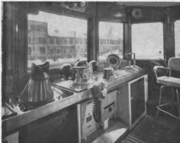
Wheelhouse has equipment conveniently located for easy use by the tug's master.
