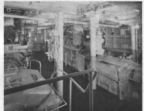
Engine room provides ample work area around Caterpillar engines and Lufkin reverse/reduction gears.
