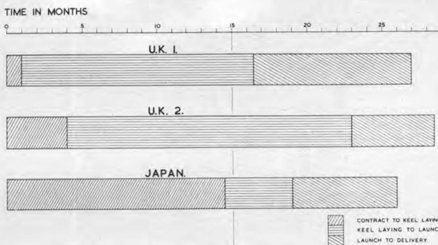
Figure 3—Comparison of building times between U.K. and Japanese shipyards.
