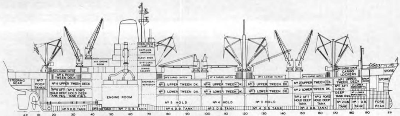
Figure 1—Inboard profile of Priam-Class cargo-liners.
