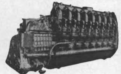
16-Cylinder Vee type—8¾ x 10½. Air starting—never run commercially. All taken from Navy D.E. vessels. You'll be surprised by the good condition of these engines. Buy now and save.
