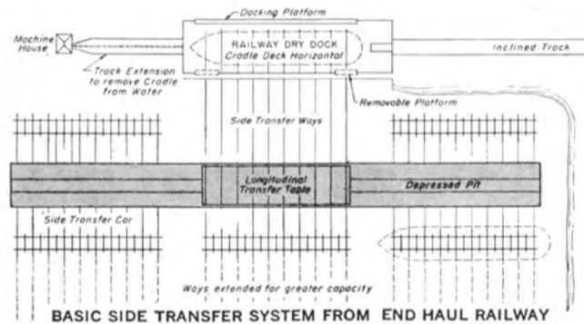
BASIC SIDE TRANSFER SYSTEM FROM END HAUL RAILWAY
