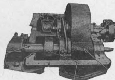
G.E. AUX. TURBO-GEN. REDUCTION GEARS Bull gear & pinion. With ABS.
