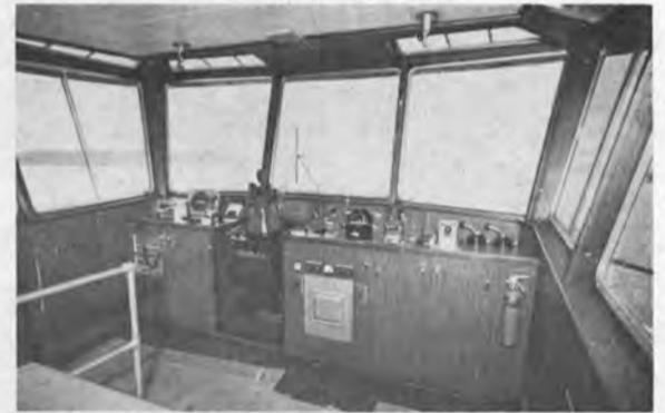
Pilothouse features overhead windows for view of ships when performing docking operations.
