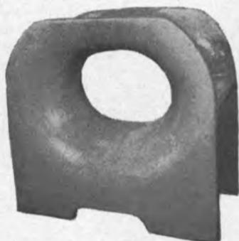
Clear opening 10" x 14" — 7" radius — with extended legs for welding to deck. Use as double or single bow chock. OAL 28" on base — OAW 14" — OAH 27 3/4" — Cast Steel.
