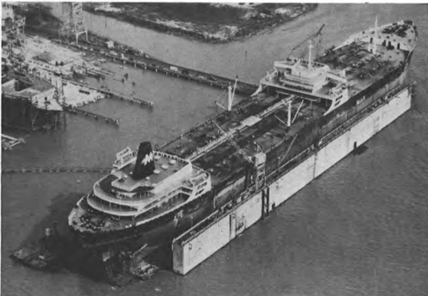
38,000 ton floating dry dock; Chester, Pa. Crandall-Type hull design reduced dead weight 800 tons
