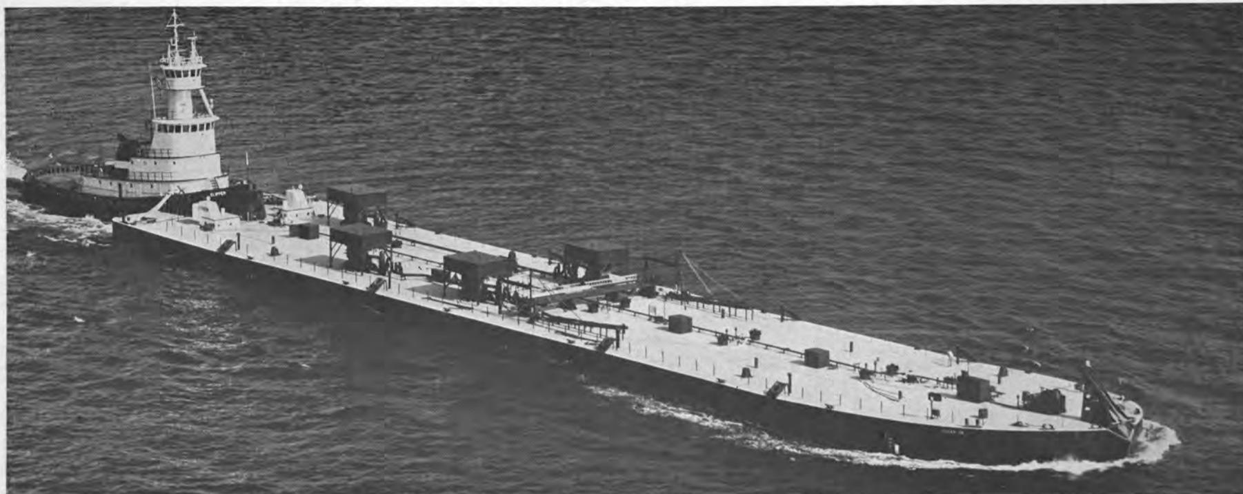
The upper pilothouse on the tug Clipper, serviced by an elevator, permits a clear view over the bow of the 16,200-dwt super-barge 135.
