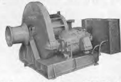
(16) single gear—single drum—7200 lbs. @ 125 FPM. MOTOR: 35 HP—230 VDC—480 RPM—compound—1/2 hour duty. Electric Brake and all controls.
