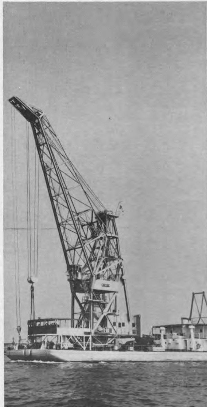
floating crane, capacity 120 tons, full slewing, self-propelled
