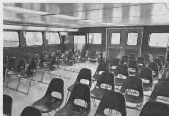
Main Salon: seating capacity 56 passengers. Passenger compartment is completely soundproofed, air-conditioned and paneled with fire-retardant Marlite. Large double doors aft provide for fast boarding and exit.
