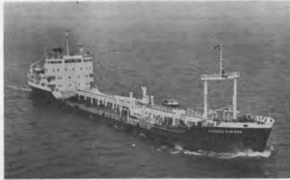
The 412-foot Ludger Simard is equipped with a steel belt at the waterline for winter navigation. Her stern bears the characteristic lines of an icebreaker.
