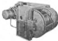
440/3/60—with controls & Stearns magnetic brake. Drum 14" diam. for 450' ¾" wire rope. Single line pull 10,000 lbs @ 450 FPM. Mfg. by Lakeshore.
