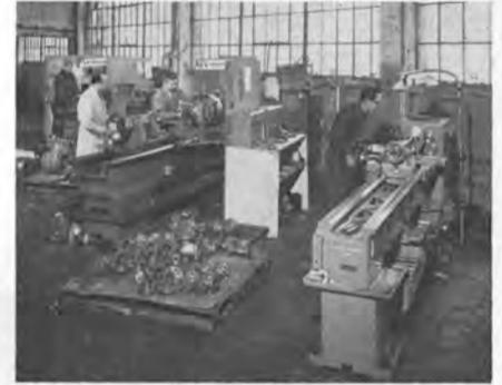
One of Zidell Valve Division's two machine shops. These shops are staffed with expert machinists to perform trim changes, modifications, surface conditioning, and reprocessing on an assembly-line basis.
