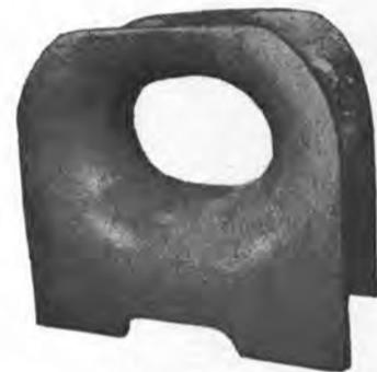
Clear opening 10" x 14" — 7" radius — with extended legs for welding to deck. Use as double or single bow chock. OAL 28" on base — OAW 14" — OAH 27¾" — Cast Steel.
