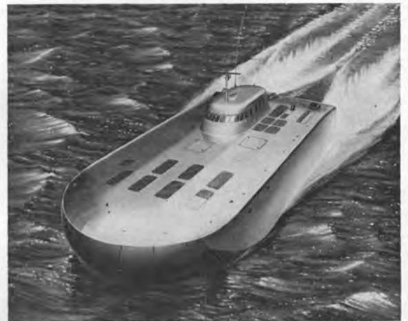
Designed for speeds in excess of 80 knots (approximately 92 mph), the hull of the test craft at times will be no more than a few inches below the water.
