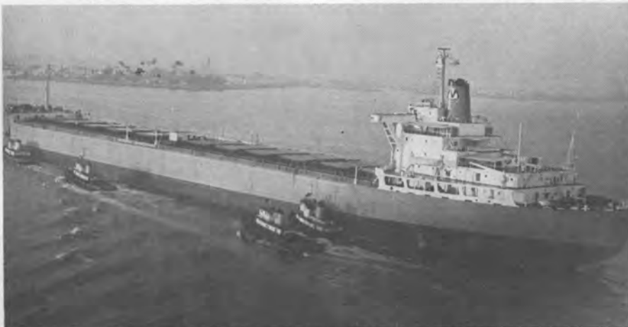
The San Juan Exporter, huge ore carrier shown above, owned by Marcona Corporation, San Francisco, will be jumboized from a present 106,000 dwt to 141,000 dwt and converted to the company's recently introduced Marconaflo slurry system.
