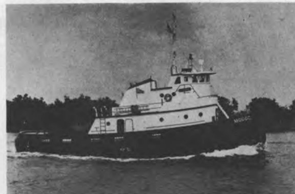
The Modoc is the second in a series of a new 86-foot Halmar class tug developed by Halter Marine Services for docking, towing and harbor operations.
