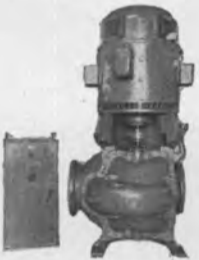
VICTORY AP2 MAIN CIRCULATOR
