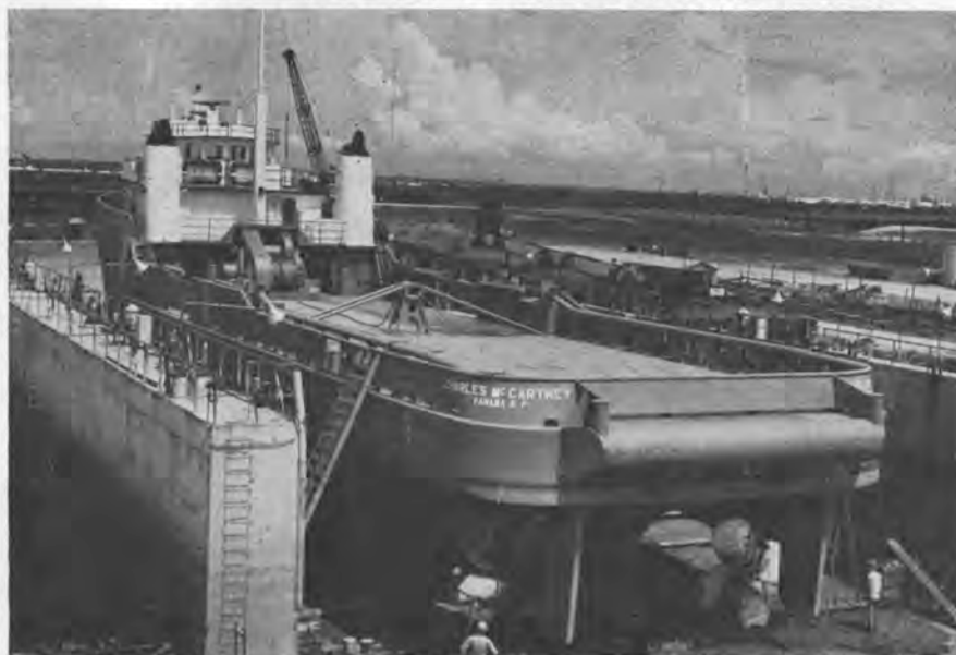
The Charles McCartney, powered by GM Electro-Motive Division diesels, has over 4,600 square feet of clear deck space for the transportation of supplies and material.
