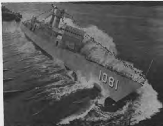
The Aylwin (DE 1081) is side launched at the Main Yard of Avondale Shipyards in New Orleans.
