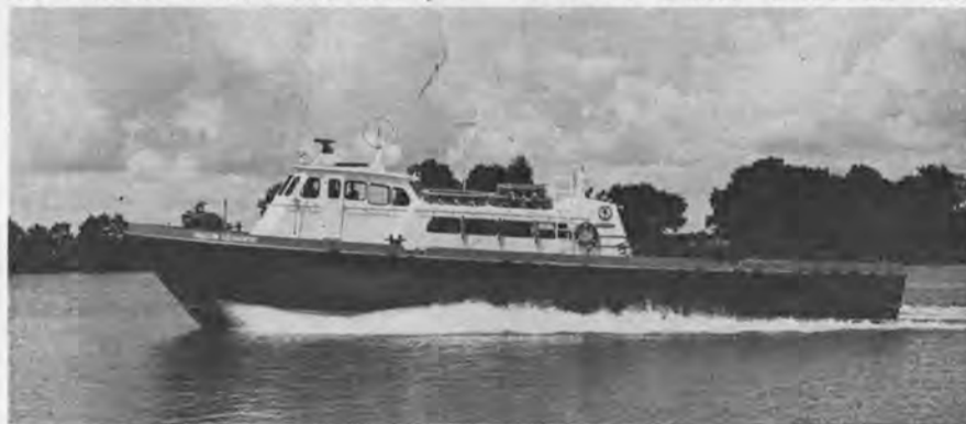
Certified to carry 48 passengers, the all-aluminum triple-screw crew boat Amazon Seahorse recorded a speed of 30 mph during her trials.
