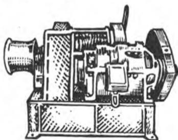
American Hoist and Derrick Company Winches with Westinghouse Motors, 50 HP, 230 Volts DC, complete with Contractor Panels, Master Switches, and Resistors.
