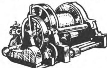
Single drum, capacity 2000' of 2" wire rope, cylinder size 9" bore by 10" stroke.
