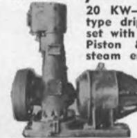
20 KW—120 volts DC—400 RPM—marine type drip-proof. Direct connected generator set with 6" x 7" bore & stroke. Type E-Plug Piston & valve—vertical self-oiling auto. steam engine. Design pressure 220 lbs—10 lbs back pressure. Complete with #62310 rheostat—wiring diagram—wrenches—terminal box & spare parts. Dry wt. 5040; shipping wt. 6300 lbs.
