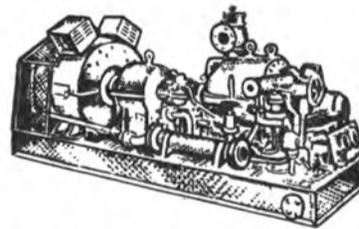
WORTHINGTON Turbines, Form S-4, 440 PSI, 740° F, with Crocker-Wheeler Generators, 300 KW, 120/240 Volts DC.
