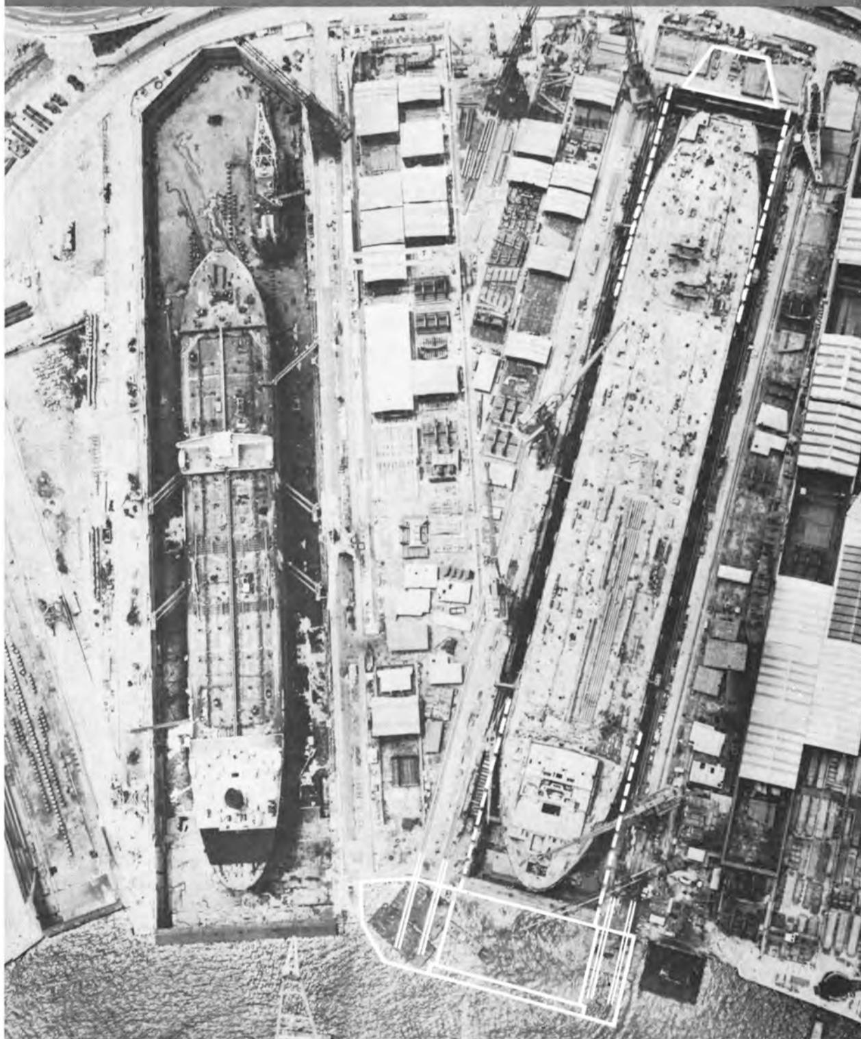
Expansion of SASEBO's present No. 4 dock of 220,000 DWT ship-building capacity to 380,000 DWT was started on September 17, 1970 to cope with the growing demands for huge tankers.
