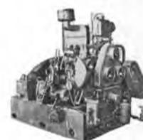
GENERATOR: Delco 10-KW—120 volts DC—83.3 amps—1200 RPM. ENGINE: Superior diesel—2 cylinder—4 1/2 x 5 3/4—15 HP—heat exchanger cooled.
