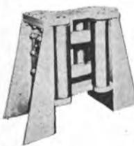
6 Rollers—2 horizontal—4 vertical. For fairleads in all directions; in-board & outboard. Strong construction, easy to maintain. Fulfills all requirements of St. Lawrence Seaway, etc. Excellent for container ships. 5½" rollers for vessels to 20,000 tons. For vessels from 20,000 to 150,000 tons, series L with 7 ½" rollers. OAH 30"—OAL 30"—OAW 17"
