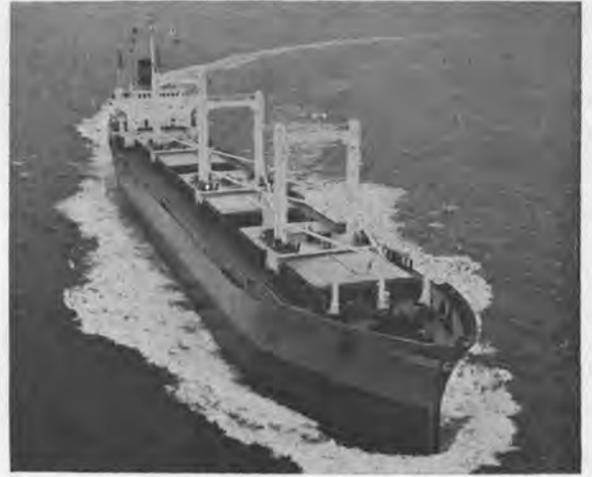
Approximate measurements of the Acritas are: 440 feet in length, 65 feet in breadth, 40 feet in depth, and a draft of 30 feet. Her main engine is a 5,130-bhp IHI-S.E.M.T. Pielstick diesel engine and provides a service speed of 13.6 knots.
