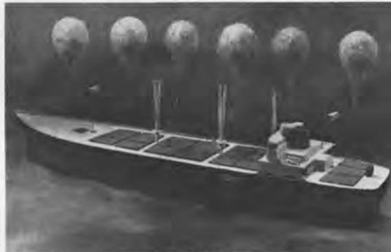
Unique salvage system shown by students at Gulf Section spring meeting uses 800,000 plastic balls pumped into the holds and six nets attached to a sunken 600-foot ship to provide negative buoyancy to raise the ship for towing.
