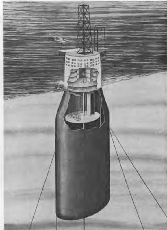
A bottle-shaped flip ship intended to revolutionize deep-sea oil drilling was designed to be towed to a drilling site in a horizontal position and then flipped to an upright position. The project was part of the third student marine-design program sponsored by Armco Steel Corp.
