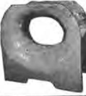
Clear opening 10" x 14"—7" radius. Use as double or single bow chock. OAL 28" on base—OAW 14 3/4"—cast steel.
