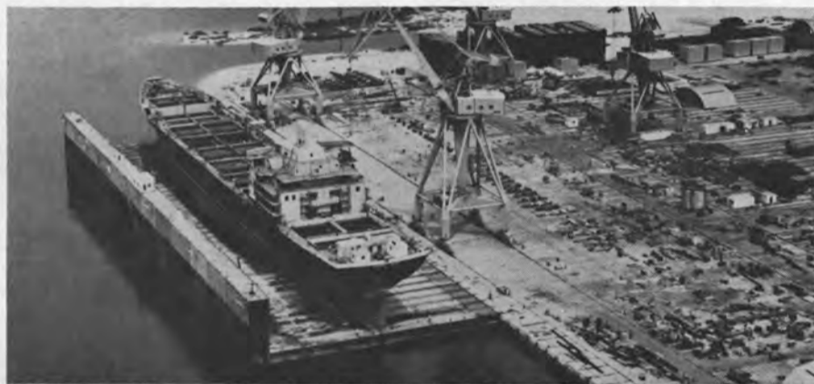
3. The Austral Envoy in its launching position on the Crandall floating dock. In this view, the portable wing-wall sections are being put in position. The platform rests on an underwater foundation. At high tide the platform is dewatered and floats free so that it can be moved into the ship channel where actual launching takes place.
