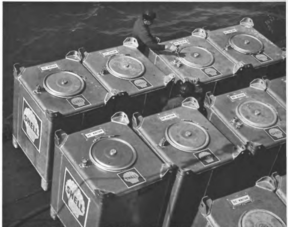
"Jumbo tanks" positioned on lighter of Standard Boat Company. Each jumbo is "dedicated"—receives only one type of oil—thus assuring freedom from contamination.
