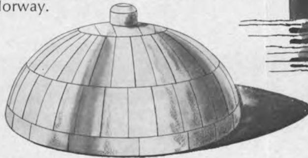
Self-supporting spherical-design tank utilizing 9% nickel steel.
