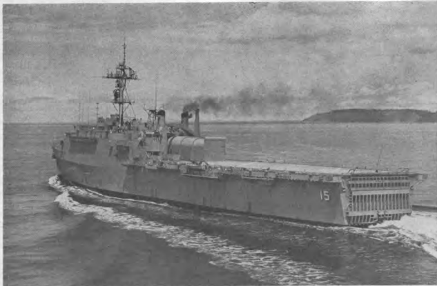
ANOTHER LOCKHEED DELIVERY: The Ponce (LPD-15) recently sailed from Lockheed Shipbuilding's West Seattle shipyard, bound for the Puget Sound Naval Shipyard, Bremerton, Wash., for commissioning. Lockheed has built seven of the large, 16,550-ton assault transports for the Navy. The ships are designed to carry 1,000 marines, their vehicles and equipment, and rush them to trouble spots to go ashore either by amphibious craft loaded in a well deck inside the ship or by helicopter from an aft flight deck. The ships are 570 feet long, 84 feet in beam, and travel at better than 20 knots. Keel for the LPD-15 was laid October 31, 1966. It was launched May 20, 1970.
