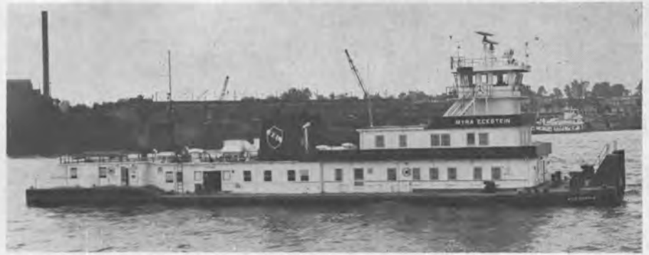
The towing knees on the Myra Eckstein, of special heavy design, provide easy access to the barges in tow at any level.
