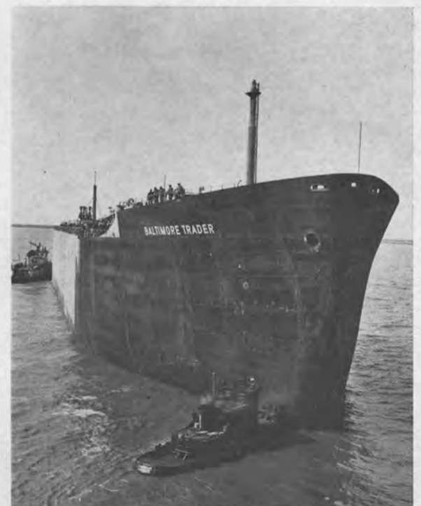
The new 625-foot forebody, which was built to mate with the 125-foot stern section, was launched at Newport News Shipbuilding and Dry Dock in March.
