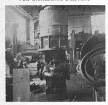
One (1) **Worthington**, 9500 GPM, 30' hd., driven by Westinghouse 100 HP, 230 V DC 800 RPM marine type drip proof motor, 20" suction, 18" discharge, all bronze—can also be furnished with AC motor.
