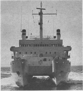
Bow view of the USNS Hayes while on trials clearly indicates the hull form. The forward lines are asymmetric while the stern lines are symmetric. This hull form was selected after extensive model testing by the Navy.
