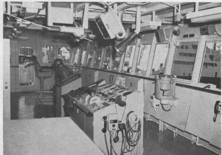
The large pilot house is fully equipped for the ship's specialized mission. Shown in the foreground is the CRP-propeller control console. This unit is duplicated at the secondary ship-control station located in the starboard quarter-deck house.
