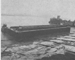
Resting in shallow water at the foot of the launching ways at St. Louis Ship's Mississippi River Yard is one of eight new Union Carbide chemicals-carrying barges. The unmanned, double-skin barges each have six stainless steel cargo tanks inside.
