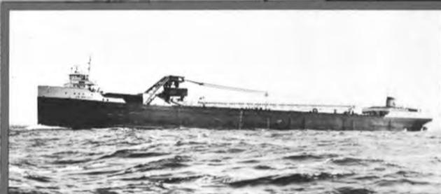
**J. R. Sensibar** Owned and operated by Columbia Transportation Division of Oglebay Norton Co., the 11,300 ton J. R. Sensibar was repowered May, 1960 with a Nordberg Marine Diesel. This engine is rated 3,200 b.h.p. at 515 r.p.m.—drives through an 800kw. generator to a single Western Reduction Gear with Wichita Clutch to a controllable pitch propeller turning at 155 r.p.m.
