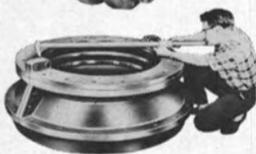
**RUDDER STOCK MARINE SEAL** . . . split construction allows installation without removal of rudder stock. A set of upper and lower seals can be supplied with lubrication system components. Upper seal has inflatable ring. Marine bronze housing. For shaft diameters of 6" and up.
