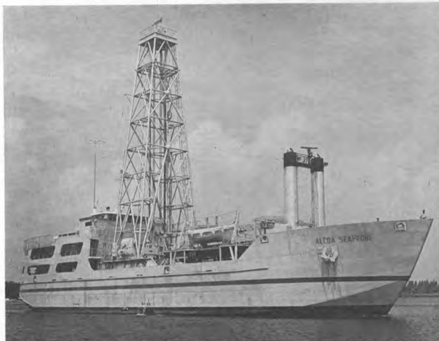
Alcoa Seaprobe on builder's trials performed in excess of planned requirements. This all-aluminum vessel not only introduced new techniques in construction methods but its capabilities for research exceed those of any existing or proposed vessel.
