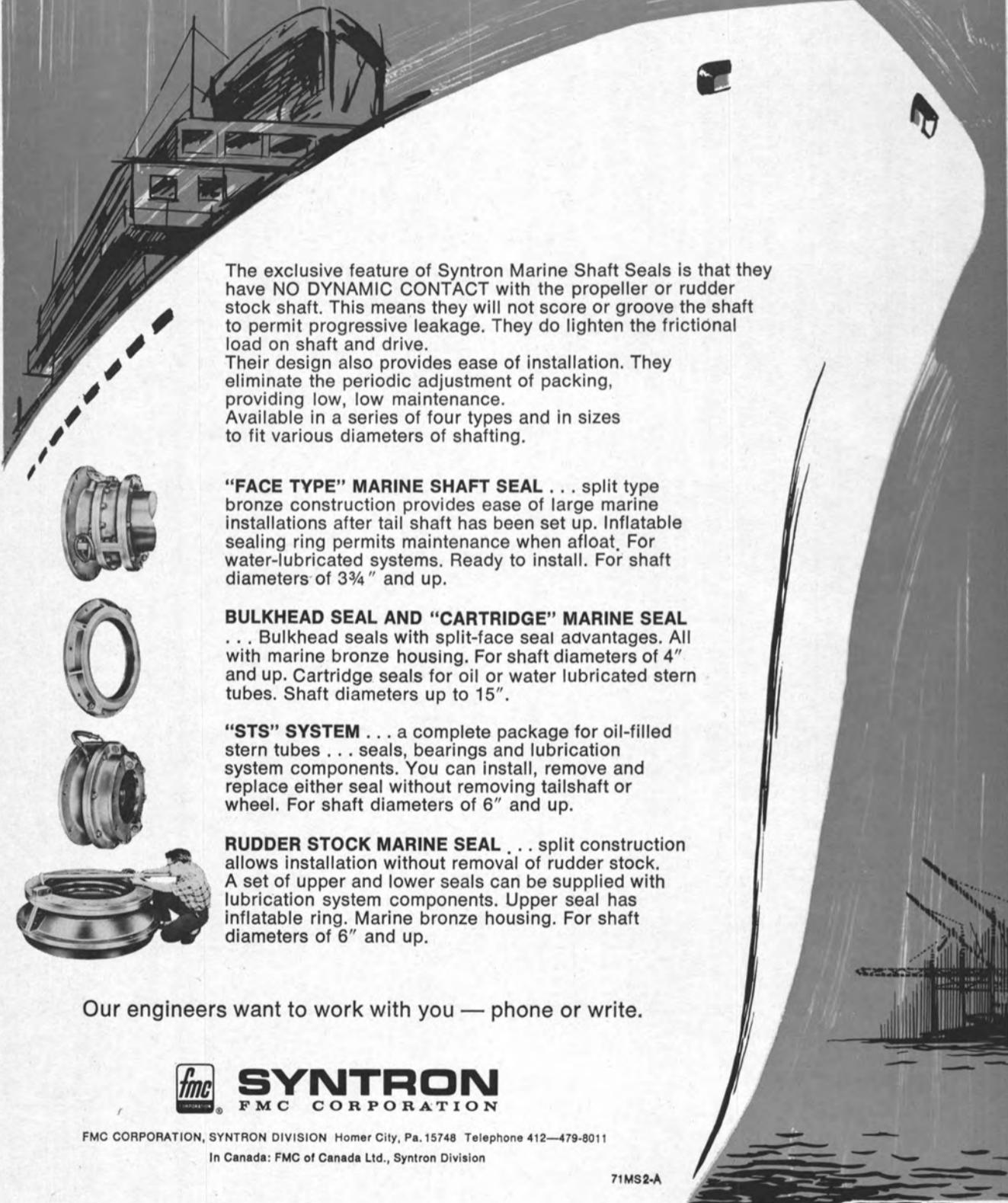
The exclusive feature of Syntron Marine Shaft Seals is that they have **NO DYNAMIC CONTACT** with the propeller or rudder stock shaft. This means they will not score or groove the shaft to permit progressive leakage. They do lighten the frictional load on shaft and drive.
