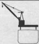
30-Ton Ship or Barge Mounted Container and General Cargo Crane.
