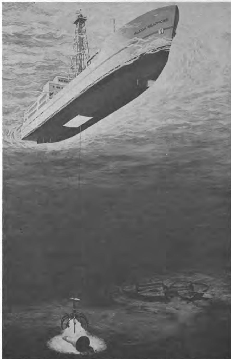
This artist's sketch depicts how the Alcoa Seaprobe will be able to recover objects 6,000 feet down and weighing as much as 200 tons. The ship possesses the capacity to remain almost stationary above a target on the bottom of the sea, and then to lower a string of pipe which will support and power coring or drilling equipment, or search and recovery gear.
