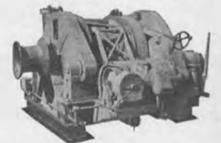
3—ALMON A. JOHNSON Stern Anchor Winches as removed from LST vessels, line pull rating 100,000 pounds at 10 FPM in low gear, complete with Contractor Panels, Resistors, and Master Switches.
