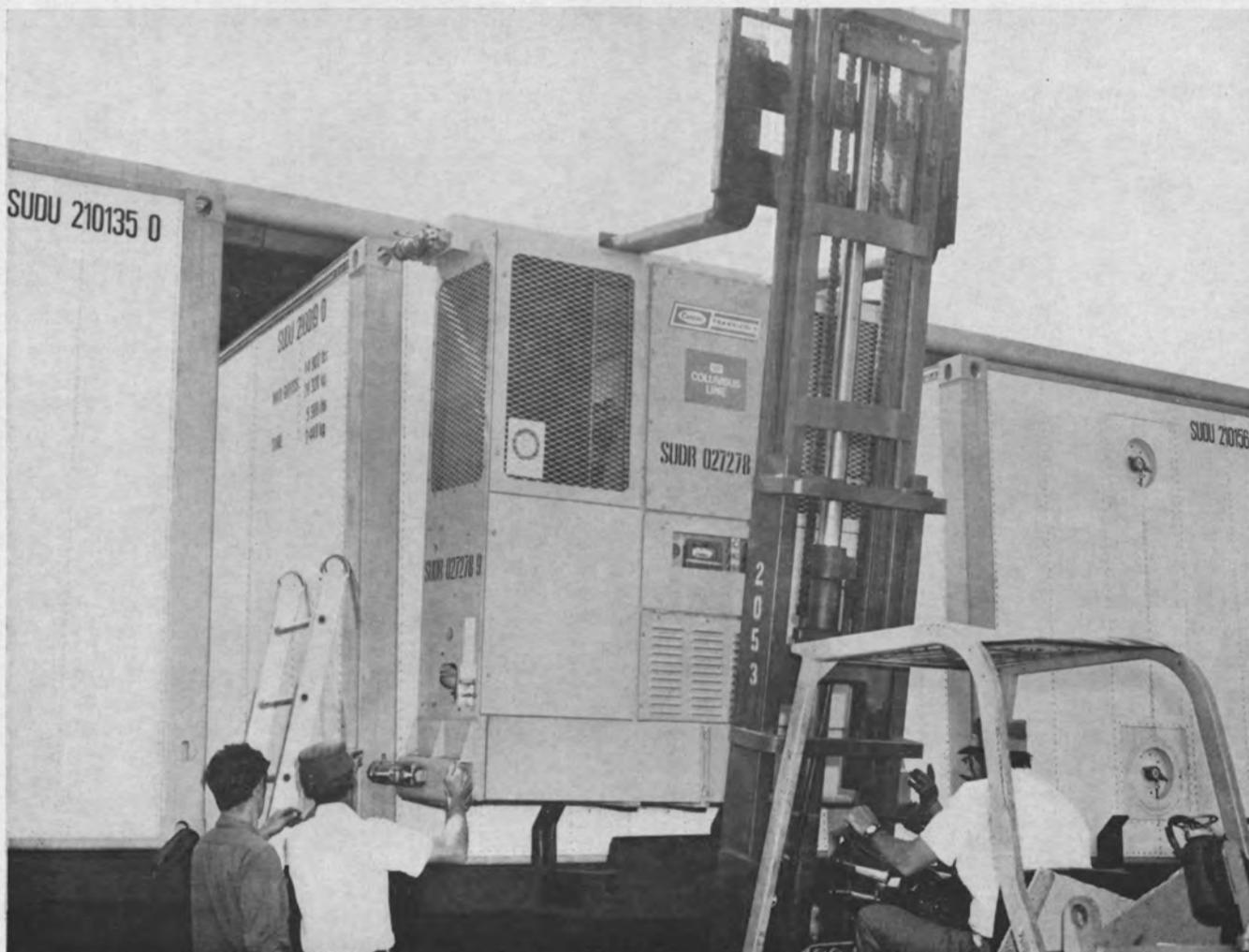
69NK simply clips to the container for shore duty, using the same air connections as aboard ship.
