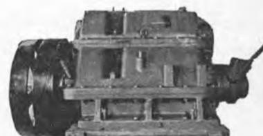
6—FALK Reverse Reduction Gears, 3 port, 3 starboard, as used with GM 12-567A Engines on LST vessels, ratio 2.48:1 ahead, 2.52:1 astern.
