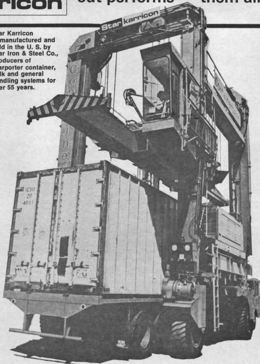
Performance records for Star Karricon in European and United Kingdom ports have proved its leadership as the most efficient straddle carrier around. It boasts an unbelievably fast average container handling cycle of 2½ minutes at a distance of 500 yards. For minimum ship turnaround time and maximum profitability, its got to be Star Karricon. Here's why:
