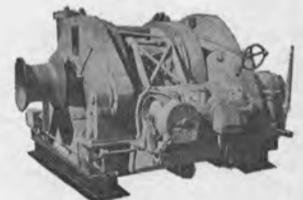
3—ALMON A. JOHNSON Stern Anchor Winches as removed from LST vessels, line pull rating 100,000 pounds at 10 FPM in low gear, complete with Contractor Panels, Resistors, and Master Switches.
