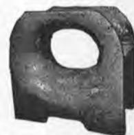
Clear opening 10" x 14"—7" radius. Use as double or single bow chock. OAL 28" on base—OAW 14 3/4"—cast steel.
