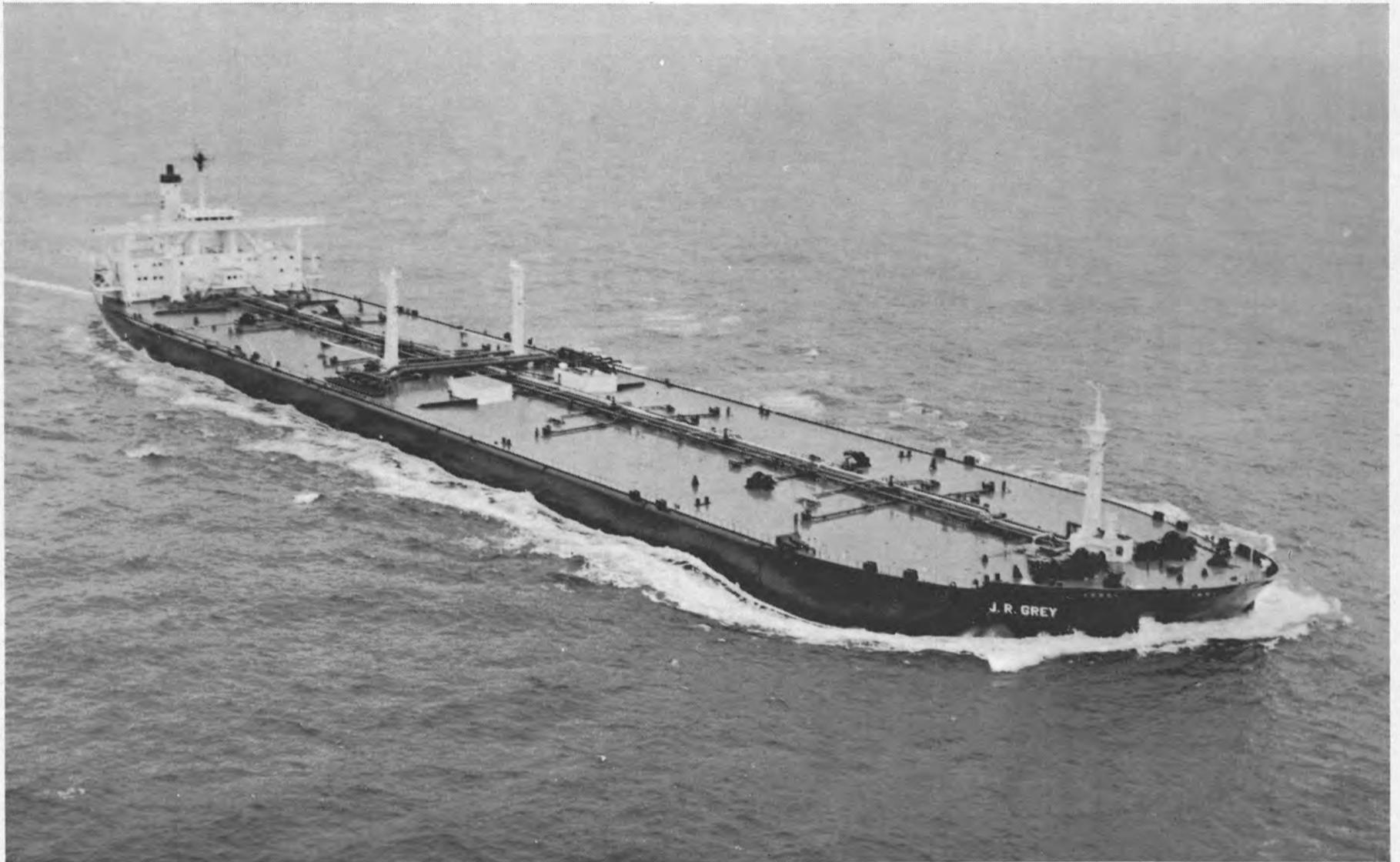
"J. R. Grey" is the second vessel of our new series of economical 260,000-dwt tankers with standardized design. The first one, the 263,231-dwt "Paul L. Fahrney" was delivered early this year. We have already received orders for 20 vessels in this class; and to facilitate fast construction, we are building the world's biggest dock at the Koyagi Works of the Nagasaki Shipyard, where the vessels are built.
