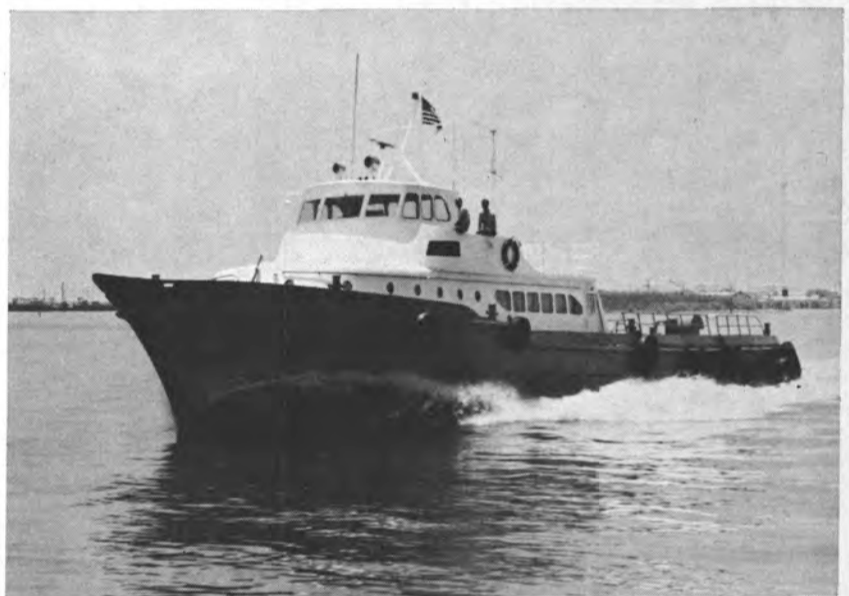
GRANDEUR: 100 ft. steel hull crewboat owned by Robin Boat Rental, Harvey, Louisiana; two Caterpillar D348 diesels; 25 mph.
