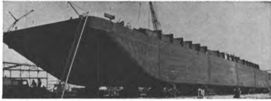
Double-Skin Chemical Barge for Inland Service
