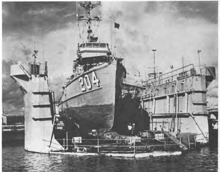
MINESWEEPER GETS A LIFT: The U.S.S. Thrush, U.S. Navy minesweeper, is shown being raised by a new 1,000-ton capacity drydock put into service recently by TRACOR/MAS Shipyard, Port Everglades, Fla. The conventional floating drydock, built by the U.S. Navy and leased by TRACOR/MAS, augments the yard's 4,200-ton capacity Syncrolift drydock and transfer system, itself one of the largest in the U.S. TRACOR/MAS officials believe this new drydock will justify a larger, more stable work force and allow more effective work scheduling and work force utilization.
