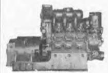
ENGINE: G.M. 6-278—6-cylinder—2 cycle—8 3/4 x 10 1/2—750 RPM—with oil and water Ross Shell and Tube Heat Exchangers, instrument panel, pyrometer, etc. Vibro Isolators. GENERATOR: G.E. 300 KW—120/240 volts DC—1250 amps—shunt wound—continuous overload rating 375 KW—2 hours—55° Weight of unit approximately 26,000 pounds. Complete with shock mounts. Unit 13' 2" long, 64" wide, 8' high.
