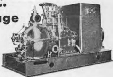
4-1250 KW, General Electric. Turbines: Type FSN, 525 PSI, 7938 RPM. Generators: 1250 KW, 450/3/60, 3600 RPM, Type ABT2.
