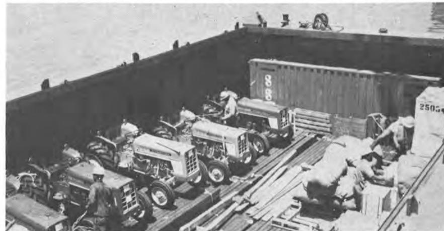
Farm tractors, long hollow steel shapes, 20-foot container, sacked cargo behind which Beefeater's gin was transported, and machinery parts are just some of the many cargoes being transported by LASH.
