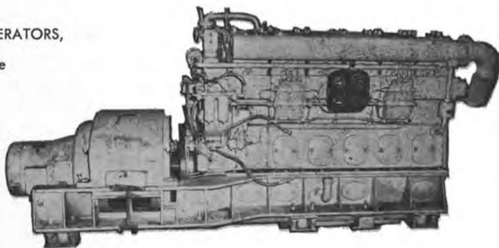
**4—COOPER-BESSEMER, Marine Model FSN6, 6 cylinders, 375 HP, 900 RPM, with General Electric Generators, 250 KW, 440/3/60.**
