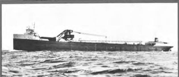
J. R. Sensibar Owned and operated by Columbia Transportation Division of Oglebay Norton Co., the 11,300 ton J. R. Sensibar was repowered May, 1960 with a Nordberg Marine Diesel. This engine is rated 3,200 b.h.p. at 515 r.p.m.—drives through an 800kw. generator to a single Western Reduction Gear with Wichita Clutch to a controllable pitch propeller turning at 155 r.p.m.
