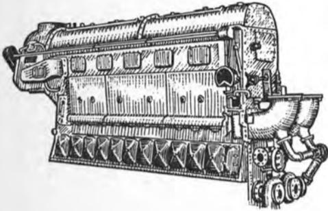
**MATCHED PAIR . . . FAIRBANKS MORSE MODEL 38D8-1/8**—1 Port; 1 Starboard. Used condition, 1800 HP, 800 RPM, 2 cycle, 8 1/2" bore, 10" stroke, Air Start. Complete with Westinghouse Reduction Gears, 2.216:1 ratio—with Hydraulic Coupling.
