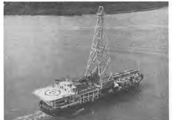
Self-propelled drill ship
