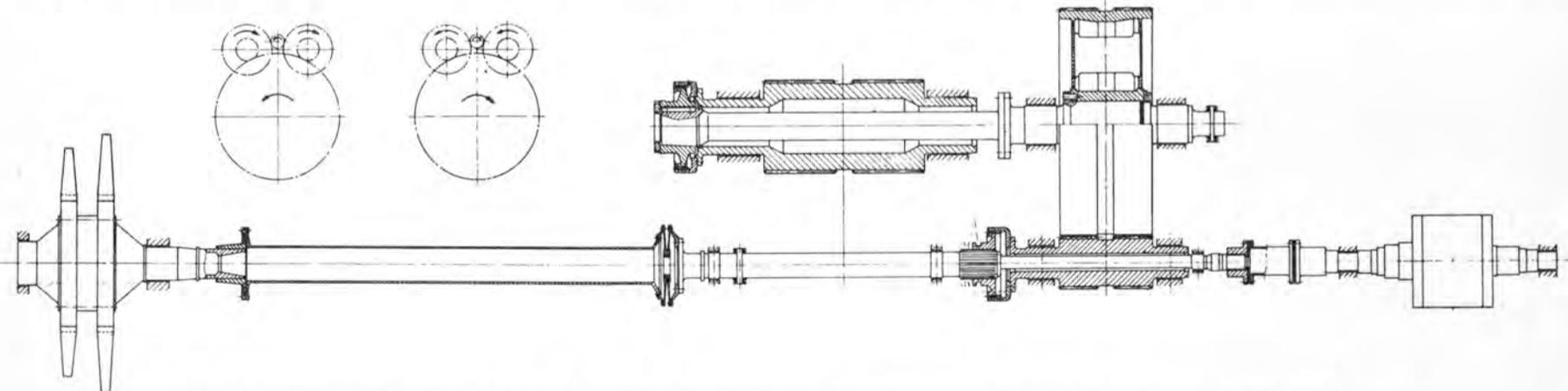
Figure 2—Layout of the high-speed elements and gearing transmission rotating parts for the Euroliner-class containerships built in Germany.
