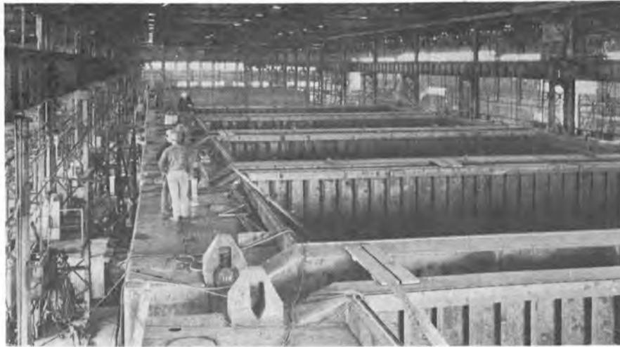
Ten LASH barges each week are completed, under cover, on this production line at Equitable's New Orleans yard.
