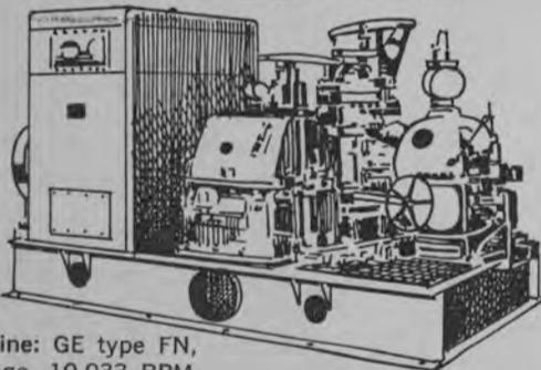
Turbine: GE type FN, 6-stage, 10,033 RPM.
