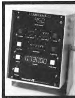
The digital indicator reads out directly in pounds. Both visual and audible alarms and an automatic tare adjustment are standard features. As an option, a boom angle digital readout can be included in the same indicator package.
