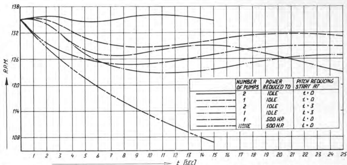
Figure 1—Computer simulations of revolutions per minute versus time for various rates of pitch change and control.
