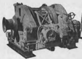
2—ALMON A. JOHNSON Stern Anchor Winches as removed from L.S.T. Vessels, line pull rating 100,000 pounds at 10 FPM in low gear, complete with Contractor Panels, Resistors, and Master Switches.
