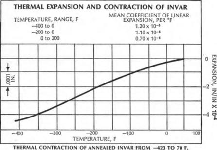
**4. Its uniformly low coefficient of expansion (.000008 in./in.)** makes Invar the ideal choice for mammoth tankers. Invar meets all API and ASME codes for cryogenic service.
