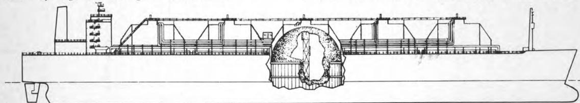
Figure 3—The 125,000-cubic-meter LNG ships have been designed by General Dynamics for the maximum standardization of the production process and flow. Unique methods have been developed for manufacturing the aluminum
