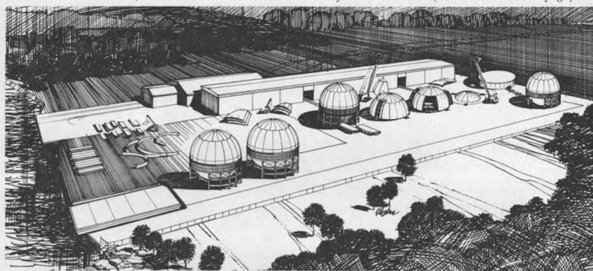
Figure 2—The proposed manufacturing plant with separate areas for the forming and trimming of plates, subassembly of sphere sections and final assembly. At the plant, the spheres will be loaded onto the barges without the use of lifting equipment.
