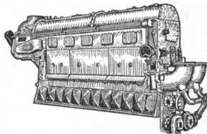
MATCHED PAIR . . . FAIRBANKS-MORSE Model 38D8-1/4—1 Port; 1 Starboard. Used condition, 1800 HP, 800 RPM, 2 cycle, 8 1/2" bore, 10" stroke, Air Start. Complete with Westinghouse Reduction Gears, 2.216:1 ratio—with Hydraulic Coupling.
