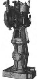
Turbine-driven main lubricating oil pumps—vertical rotary with horizontal worm geared turbine drive. 575# Steam pressure—5000 RPM—1.5# back pressure. GEAR: 5000/1035 RPM. PUMP: 550 GPM at 50 PSI—suction lift 10.0". Suitable for Fletcher Class Destroyer.
