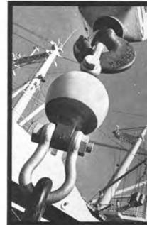
Since the Load Transmitter is completely wireless and simply "hangs" on the end of the hook block, it doesn't affect the crane's rigging in any way. And it can be transferred from one crane to another or from the main to the auxiliary hook block on the same crane — in less than ten minutes.
