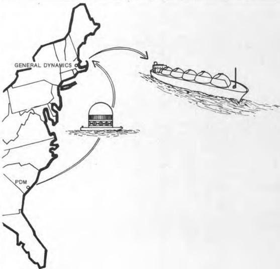
Figure 4—The finished LNG spheres will be shipped from the manufacturing plant to Quincy by barge. At the yard, the spheres will be unloaded and placed into the ship's hull using a unique 850-ton-lift crane especially designed to handle the spheres.
