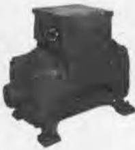
INPUT: 115 VDC—6.1 amps—3600 RPM. AC OUTPUT: 425 watts—110/1/60. Ball bearing, 13 7/8" long—7 9/16" wide—10 1/2" high. Has radio noise suppression filter. Net wt. 58 lbs—83 lbs packed for shipping.
