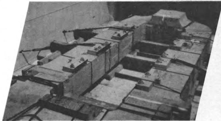
Electrical machinery heavy lift (142 L.T.) is secured in LASH barge for export.
