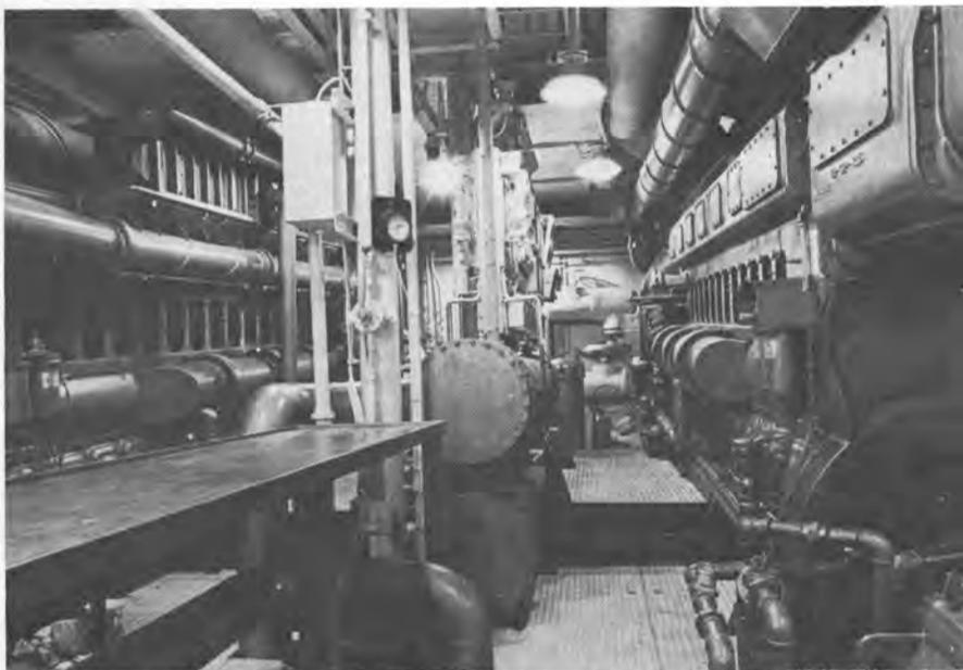
Looking forward in the engine room between the two Fairbanks-Morse diesel engines indicates ample work areas. These engines are remotely controlled from the bridge.
