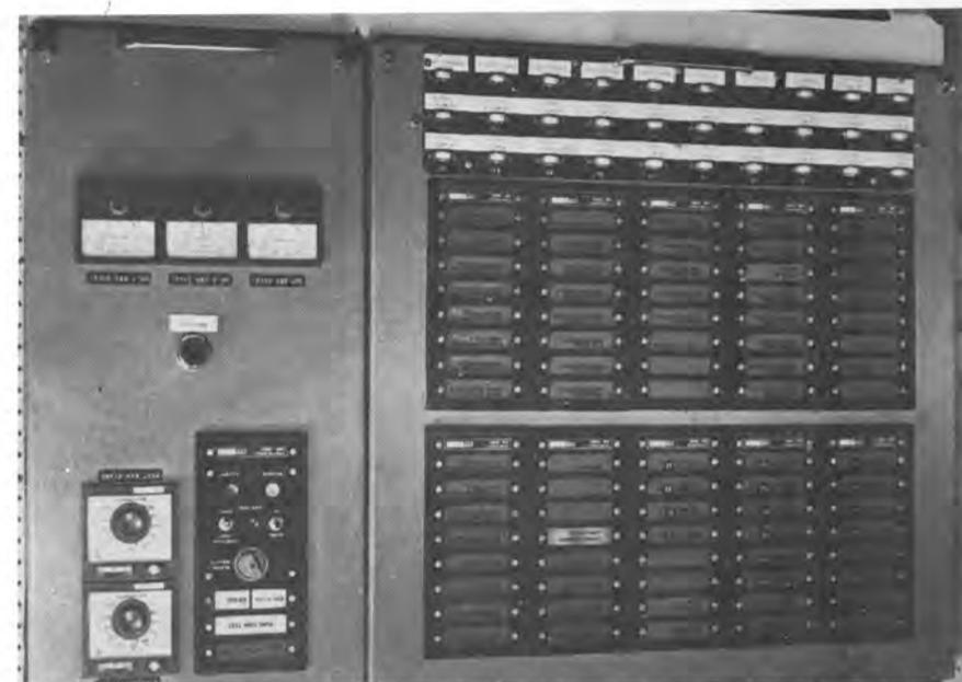
The ITT Decca Marine monitoring panel covers 76 points throughout the vessel. This system assures efficient and trouble-free operation during critical fishing.
