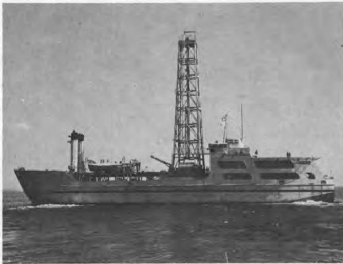
"ALCOA SEAPROBE"—The world's largest all-aluminum Oceanographic Research Vessel: Length: 243', Beam: 50', Derrick: 132' above W.L., Propulsion: Two cycloidal omni-directional propulsion units, Range: 6600 miles.
