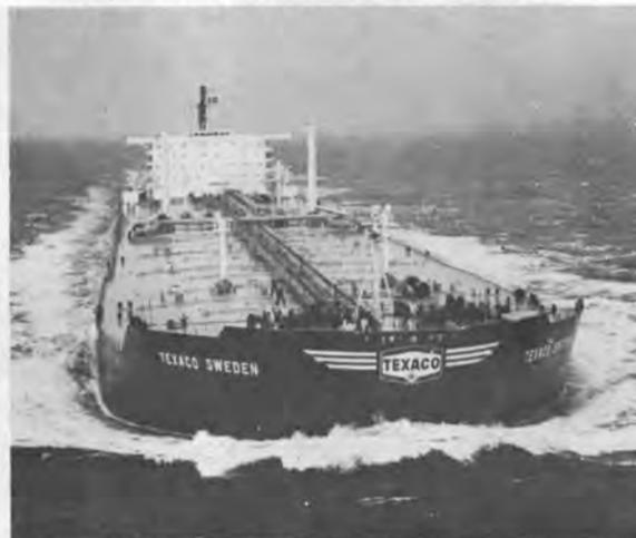
The eleventh 255,680-dwt tanker in a series of 20 such ships—the Texaco Sweden—is shown during her successful sea trials in the North Sea. Designed and built by Kockums, this class of ships has shown excellent results on trials.
