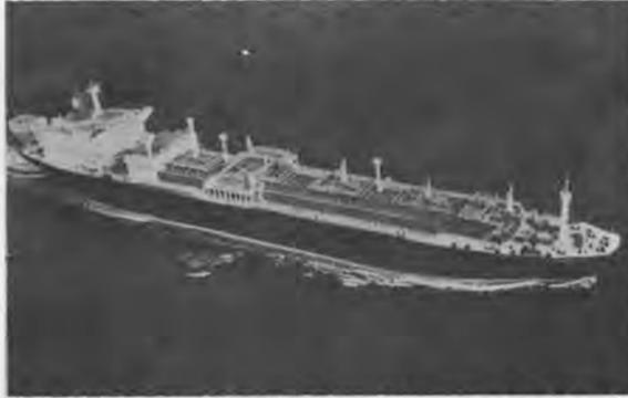
The *Gadunia*, 75,000-cubic-meter capacity, is the first in a series of five LNG tankers of the same design. All five vessels will be used to transport LNG from Brunei to Japan.
