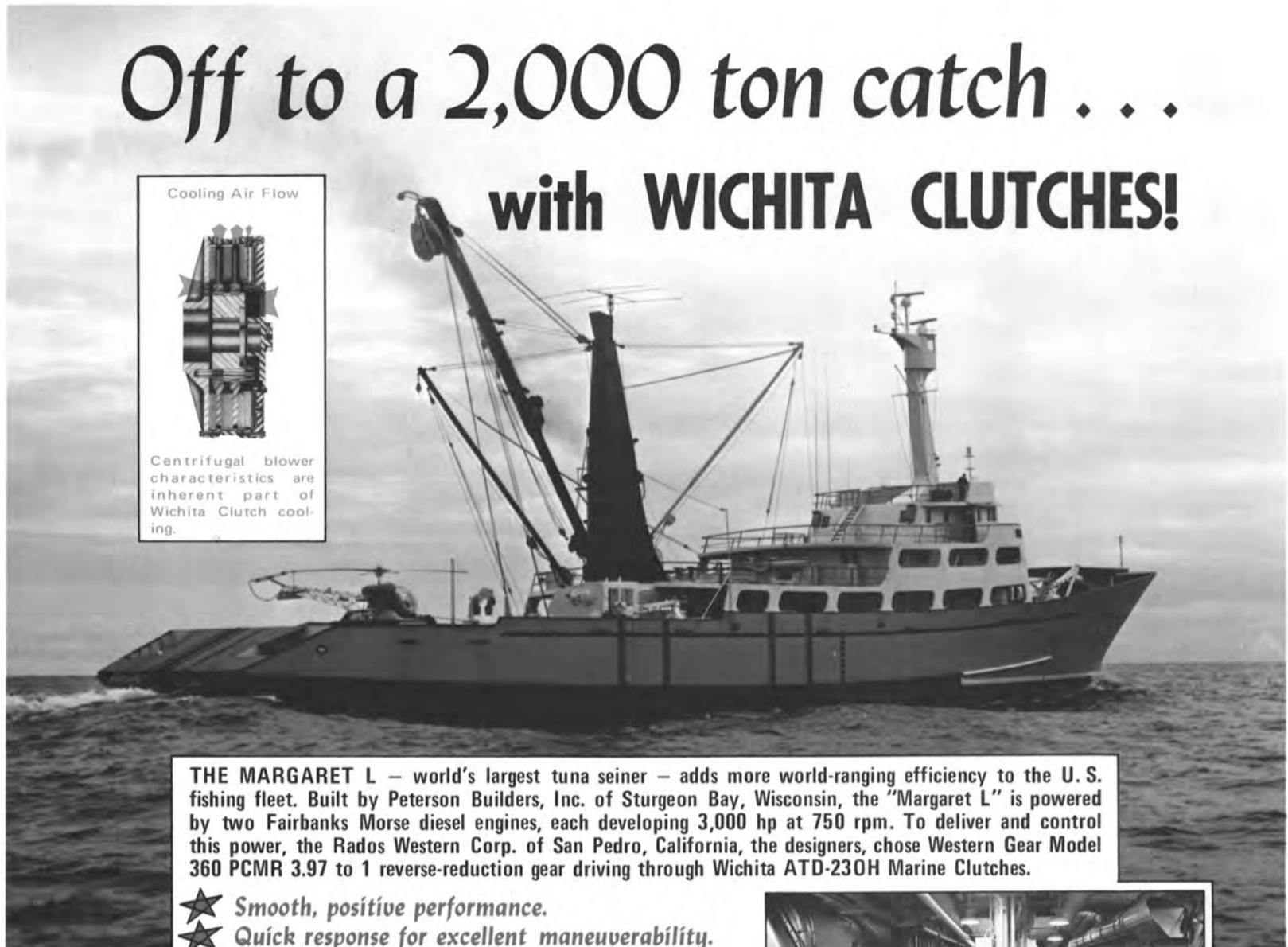
**THE MARGARET L** – world's largest tuna seiner – adds more world-ranging efficiency to the U. S. fishing fleet. Built by Peterson Builders, Inc. of Sturgeon Bay, Wisconsin, the "Margaret L" is powered by two Fairbanks Morse diesel engines, each developing 3,000 hp at 750 rpm. To deliver and control this power, the Rados Western Corp. of San Pedro, California, the designers, chose Western Gear Model 360 PCMR 3.97 to 1 reverse-reduction gear driving through Wichita ATD-230H Marine Clutches.
