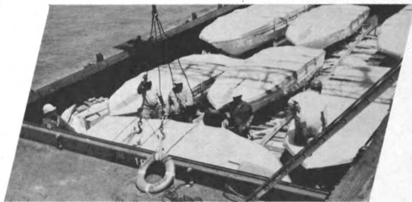
Seven 17 to 22-foot-long inboard/outboard boats are stowed over flour, carborundum, resin, machinery parts and other general cargo.
