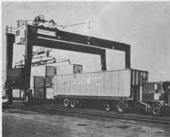
Paceco 40-long-ton Transtainer at the Port of Norfolk, Va., similar to the two Transtainers to be installed at the North Point Wharves.
