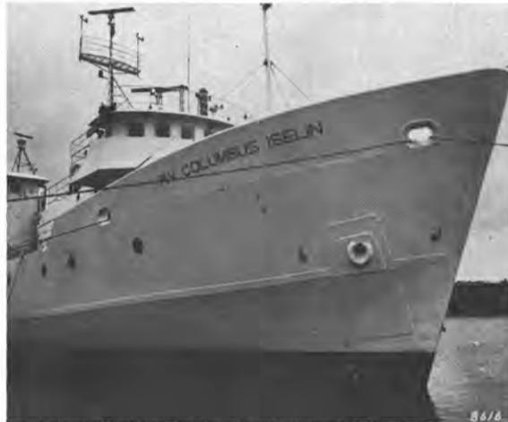
The \$1.4-million R/V Columbus Iselin, shown at dockside in the Bellingier Shipyards, Jacksonville, Fla. Forty-foot-long steel plates, supplied by Republic Steel's Gadsden, Ala., mill, were used for its construction and in the making of the molded hull.
