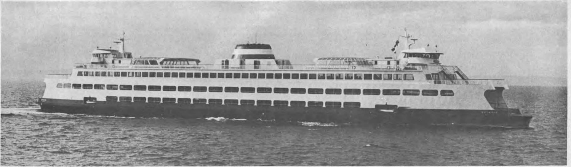
Powered by General Motors Electro Motive Division 8,500-hp diesels driving Coolidge propellers, the double-ended Spokane had to go through two complete trial tests—once for each end.
