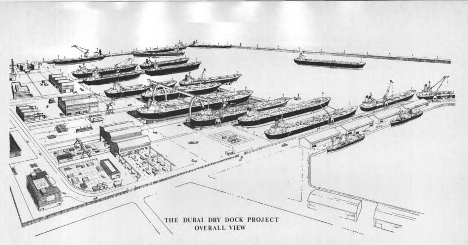
The new Arabian Gulf repair facility will have 11 berths, five moorings, three drydocks, two of which will handle vessels up to 500,000 dwt, and the third capable of handling 1,000,000-dwt tankers.
