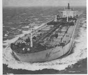
The Gotaverken-built T/T Corona has been built to the highest class of Det norske Veritas and classed EO (unmanned engine room).
