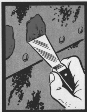
FILL PITTED HULLS
