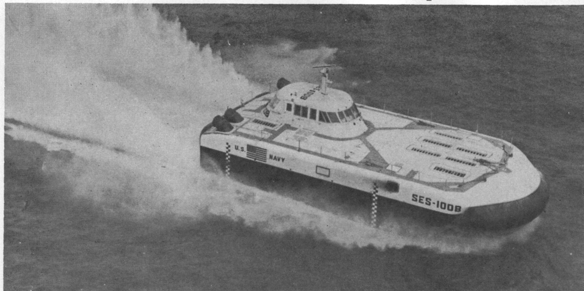
Data being collected during the SES-100B test and evaluation program is being applied to the preliminary design of a 2,000-ton operational prototype Surface Effect Ship for the U.S. Navy.
