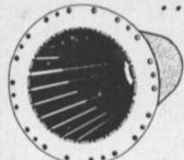
DOVETAILED BRONZE HOUSINGS WITH METAL-BACKED RUBBER STAVE BEARINGS
