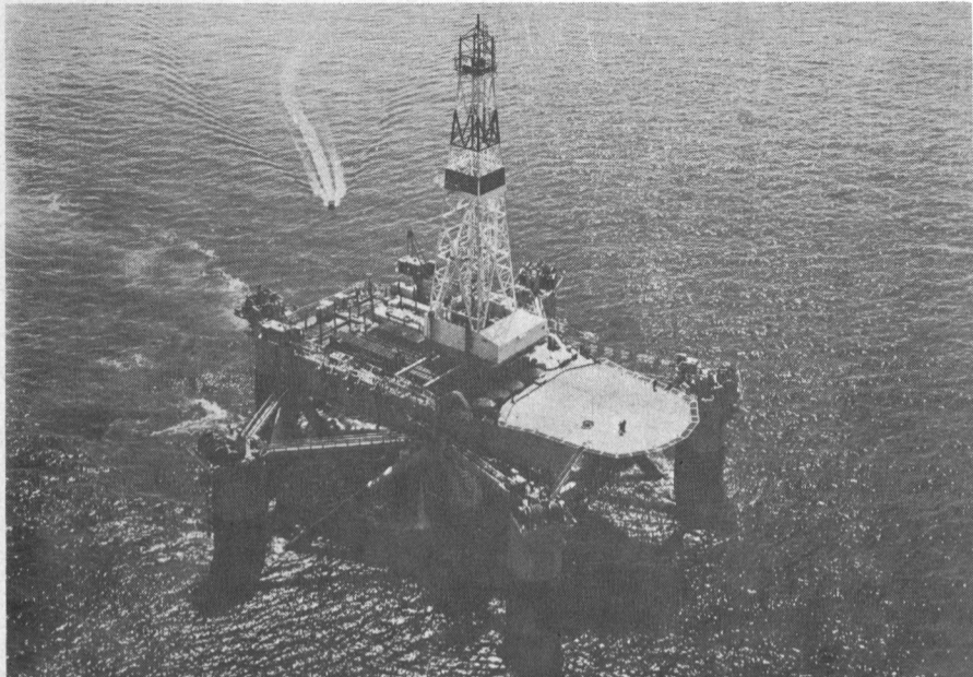
A semisubmersible drilling platform similar to the French-built Pentagone 81 pictured here is being built at Marathon's Brownsville, Texas yard for Societe de Forages en Mer "Neptune." The Pentagone 81 is a 5-column platform. The rig can drill in water depths to 600 feet, and its special design enables it to perform in rough sea environment.
