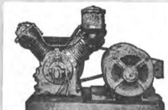
2—GARDNER-DENVER, 150 CFM, 125 PSI, Class WB, Size 7x5 3/4 x5, with Diehl Motors, 45 HP, 230 Volts DC, 870 RPM, 167 Amperes.
