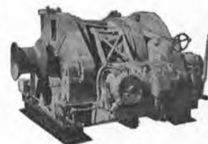
2—ALMON A. JOHNSON Stern Anchor Winches as removed from LST vessels, line pull rating 100,000 pounds at 10 FPM in low gear, complete with Contactor Panels, Resistors, and Master Switches.
