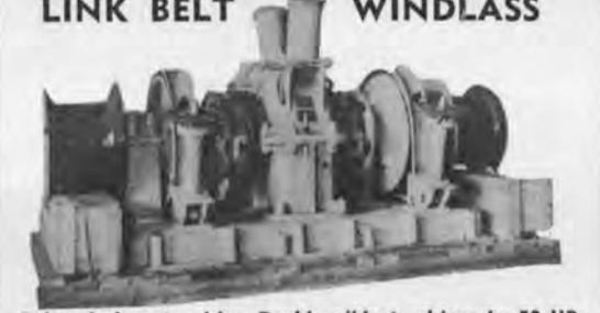
Below deck motor drive. Double wildcat—driven by 50 HP 230 VDC motor with vertical shaft and worm drive. Single speed—handles 7000 lb anchors and 60 fathoms of 1 5/8" chain at 7 fathoms per minute. Wildcat centers 56". Complete with all controls and warping features. Total weight 27,500 lbs. With spares.
