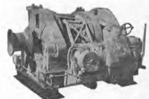
2—ALMON A. JOHNSON Stern Anchor Winches as removed from LST vessels, line pull rating 100,000 pounds at 10 FPM in low gear, complete with Contactor Panels, Resistors, and Master Switches.
