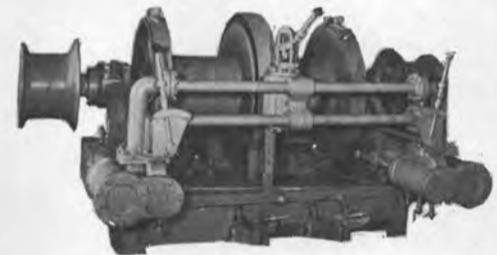
Drum 8500 lbs @ not less than 120 FPM; 13,000 lbs at no specific speed. Gypsy head 22,500 lbs static pull. Foot brake to hold 17,000 lb. pull. Steam cylinders with standard 250 PSI.
