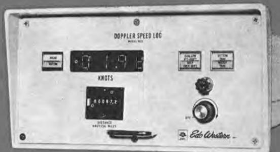
This versatile, high accuracy digital system provides precise ships speed and distance traveled information. Pulse mode and CW mode depth capabilities overlap to ensure operation in all water depths. The Model 582C is installed on vessels worldwide and boasts an impressive record of proven performance and high reliability, placing it far ahead of all other types of speed logs on the market.
