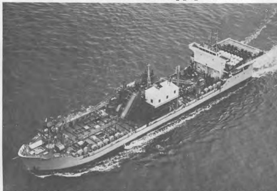
The Petrobras II leaves the Tamano yard of Mitsui upon acceptance of her owners. The self-propelled drilling rig is designed to rotate its amidships drilling rig.
