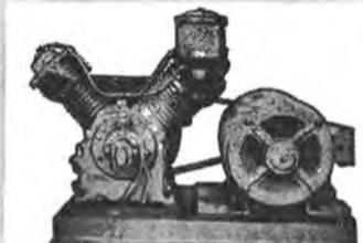
2—GARDNER-DENVER, 150 CFM, 125 PSI, Class WB, Size 7x5 3/4 x5, with Diehl Motors, 45 HP, 230 Volts DC, 870 RPM, 167 Amperes.
