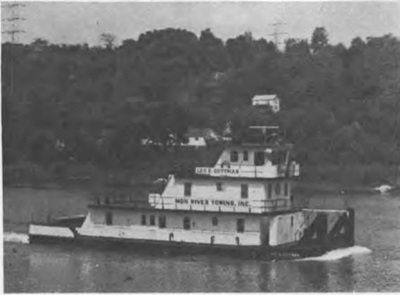
The M/V Leo D. Guttman, which provides living quarters for a crew of eight, has a pilothouse with an eye level of 24 feet.
