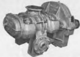
Mfg. Waterous Co.—730 GPM—pump speed 232
