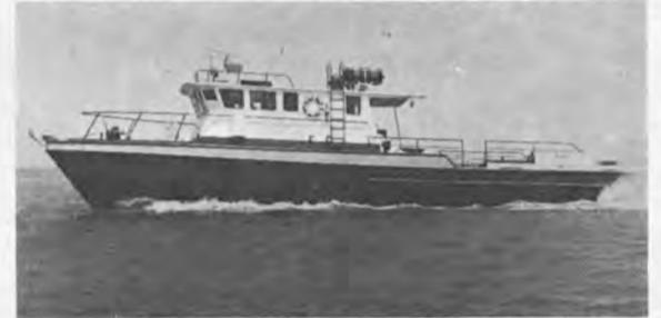
Designed and built by Halter to Lloyd's Class 100-A Nigerian Service classification, the new crewboat can accommodate 32 passengers.
