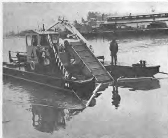
The forward throat area of the vessel incorporates a wide-angle debris deflector leading into a conveyor. The throat area can also incorporate an oil skimmer attachment.
