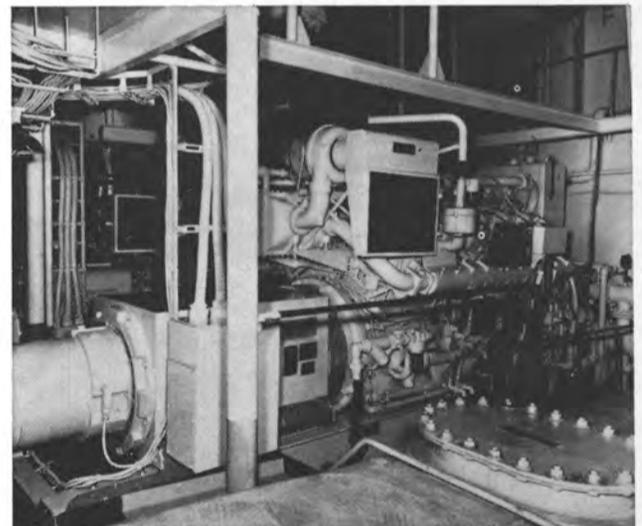
One of three VHP V12 L5790 DSIM Enginators on the "Malaspina." For ship's service power, Waukesha offers units from 47 to 1110 kw.
