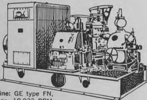
Turbine: GE type FN, 6-stage, 10.033 RPM.
