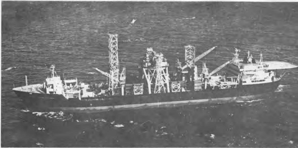
The Hughes Glomar Explorer may be conned from either the forward or aft bridge. Under normal operating conditions, the mining ship will be conned from the forward bridge while under way, and from the aft bridge while mining.
