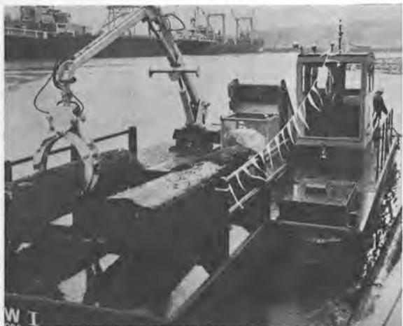
The hydraulic crane loader can lift sunken or floating objects from the throat area or from alongside the vessel and place the material on the aft deck.
