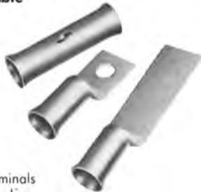
Long barrel AMPPOWER terminals and splices speed termination of stranded cable up to 1000 MCM. Barrel end of terminal is readily sealed with heat shrink tubing for maximum protection of cable against water and corrosion. Available with double thick blank or stud-hole tongue. **Circle 30 on Coupon.**
