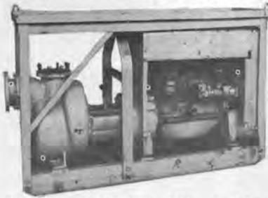
Reconditioned—mounted in portable steel frame. 1750 RPM—1100 GPM @ 100' head; 1500 GPM @ 70' head; 1800 GPM @ 50' head; 2100 GPM @ 20' head. Leroi gas engine—model D-201P3
