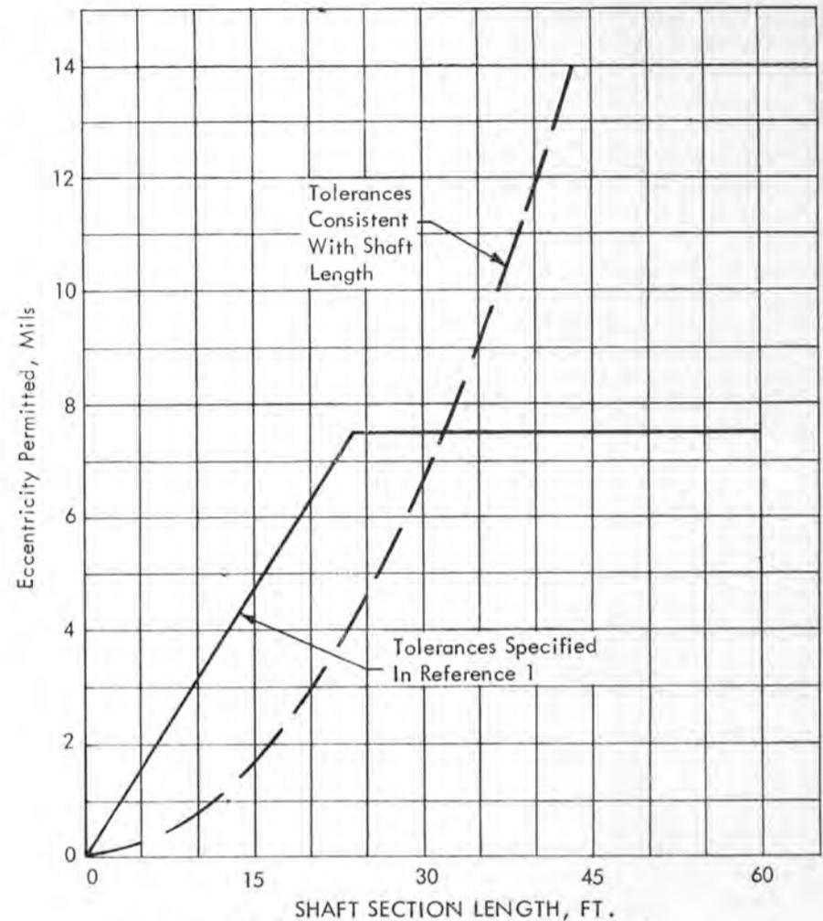
Figure 2—Eccentricity tolerances versus shaft length. (Reference 1 refers to NavShips Standard Drawing 810-2145807, July 1967)
