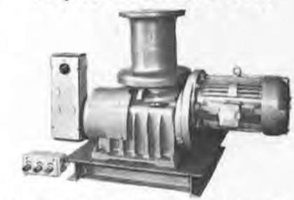
**MOTOR: 10 HP—totally enclosed—fan cooled—continuous duty—horizontal flange mounted—special shaft & oil seal fitted—440/3/60—1760 RPM. CONTROL: Marine type watertight pushbutton — forward / reverse / stop—watertight starter box—rated for 40 starts/hour—triple pole contactor with silver contacts, thermal overload relay & trip adjustment. DIMENSIONS: Barrel 10" diam.—flange 10" diam.—approx. 26" wide & 36" long.**
