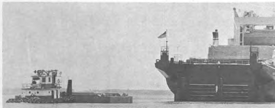
A stern view of the Delta Mar with a tug going into the slot with a lighter. The fendering system in the stern slot can be seen as well as the crane with a barge.
