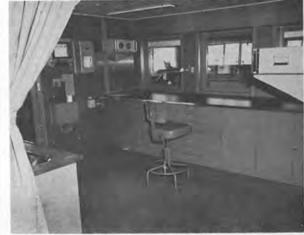
The chart room is located centrally behind the pilot house. An Omega receiver, a depth finder, wind speed and direction indicator and other instruments are in this room.
