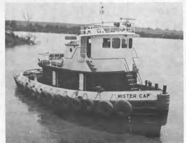
MISTER CAP JOINS F & S FLEET: Service Machine & Shipbuilding Corp. of Morgan City, La., recently delivered the M/V Mister Cap, a 1,200-hp tug, to F & S Boat Corporation, a division of Elpac, Inc. The vessel, named after F.L. Capert, chairman of Elpac's board, measures 75 feet by 24 feet and is equipped with two 16V71N engines by General Motors, MG527 clutches by Twin Disc, two 30-kw generators by Delco with G.M. 371 power, anchor handling winch (100,000# line pull), fire fighting system, and a complete package of modern electronic equipment. F & S Boat Corporation is under the management of Andy Wedaman and Albert (Sam) Smith Jr., and operates 14 tugs from offices in Morgan City and New Orleans, La., Houston, Texas, and London, England.
