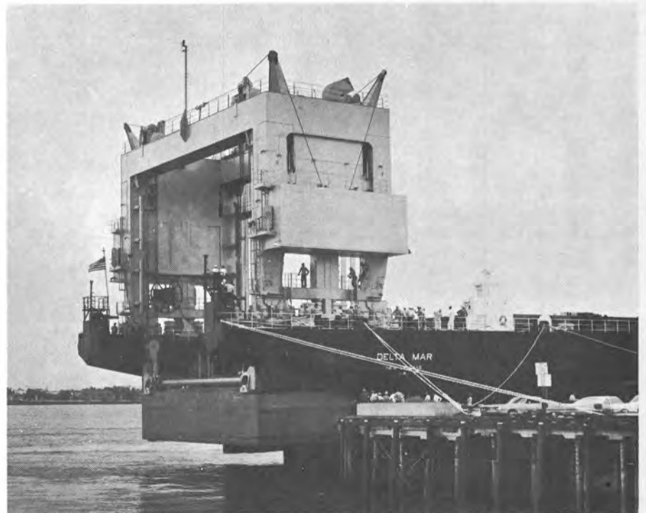
The Delta Mar taking on her first loaded barge at New Orleans in preparation for the ship's maiden voyage. The massive Morgan crane can lift and transport 455 long tons.
