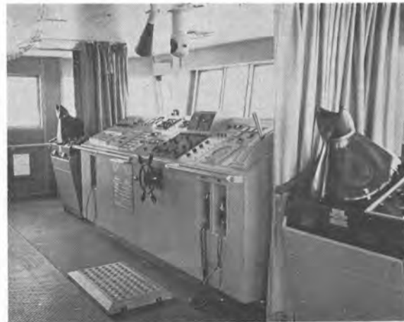
This view of the pilot house shows the bridge console with conning station, throttle control, watch call buttons, navigation lights, etc. centrally located between the radars.
