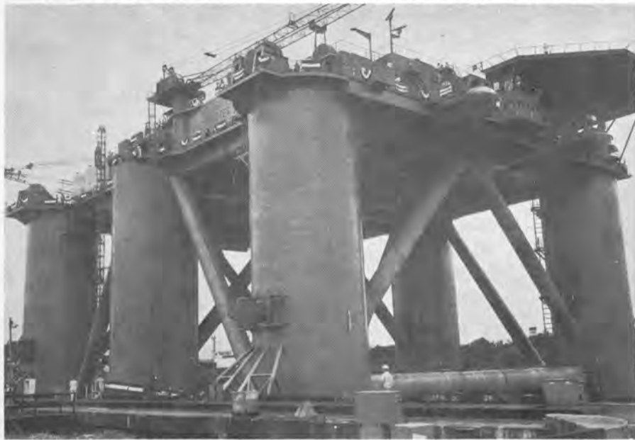
Designed by Friede & Goldman, the Pacesetter can drill in wave heights up to 30 feet.
