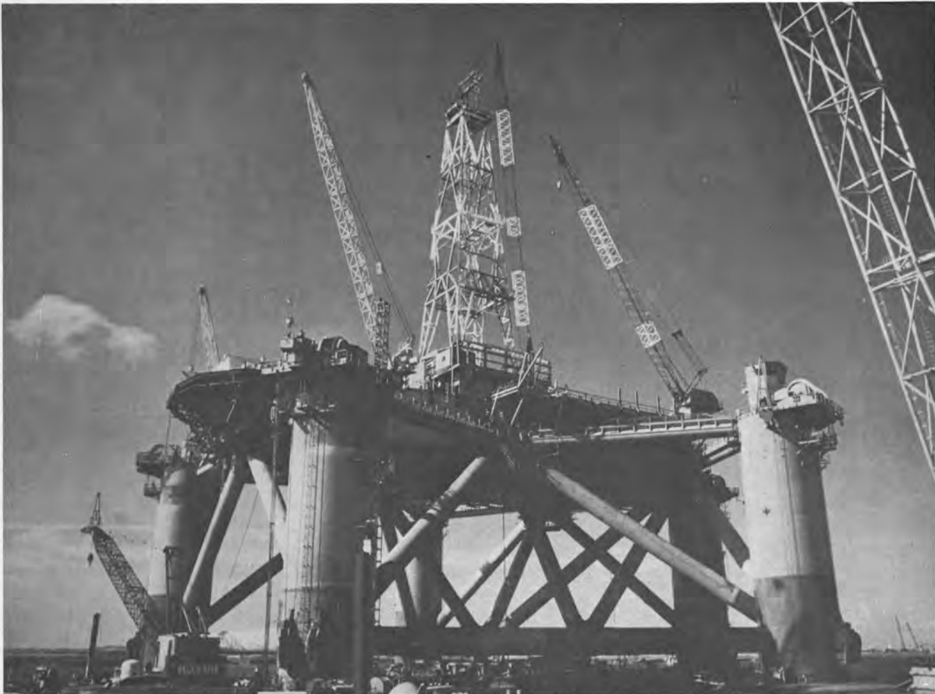
COMMISSIONING —The Pentagone 82, a semi-submersible offshore drilling rig weighing more than 10,200 tons, during the recent commissioning ceremonies at the Gulf Marine Division shipyard of Marathon Manufacturing Company, located in Brownsville, Texas.
