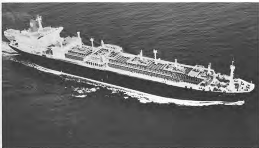
The LNG tanker Gadinia . Built by Les Chartier de L'Atlantique at St. Nazaire, France. She went into service December, 1972. She has the low silhouette characteristic of membrane tankers.
