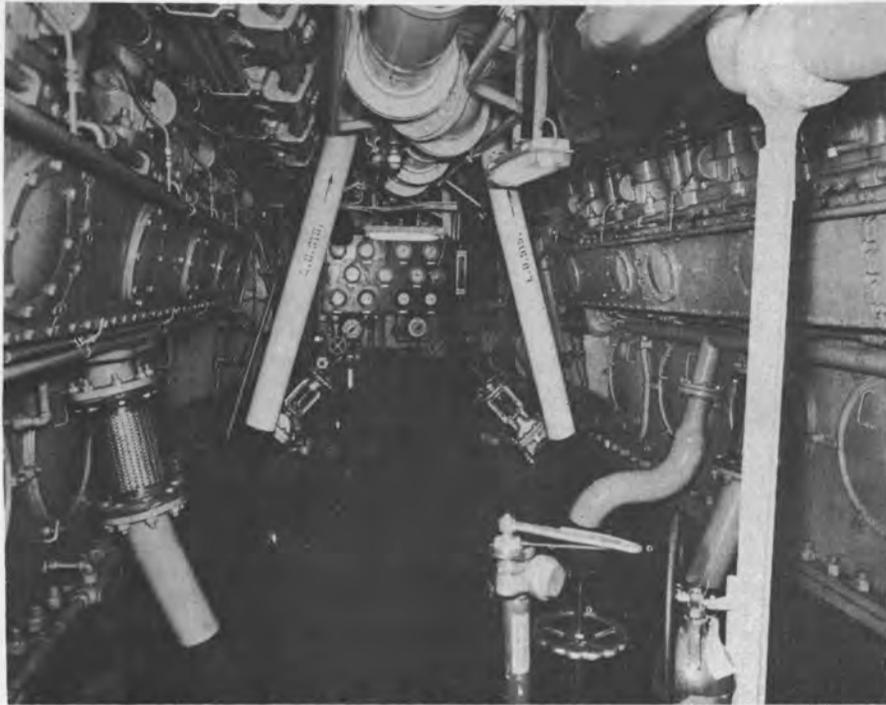
This view of the lower engine room is taken looking aft between the two Colt Diesels.
