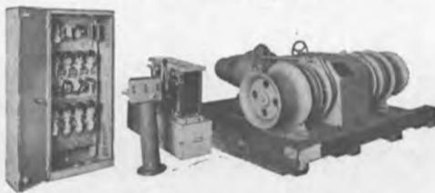
For 1-5/16" chain—on 36" centers. 15 H.P.—115 volts DC—1750 R.P.M.—6000 lb. line pull.
