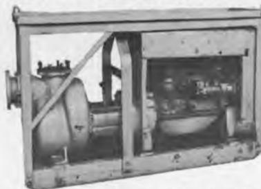
Reconditioned—mounted in portable steel frame, 1750 RPM—1100 GPM @ 100' head; 1500 GPM @ 70' head; 1800 GPM @ 50' head; 2100 GPM @ 20' head.
