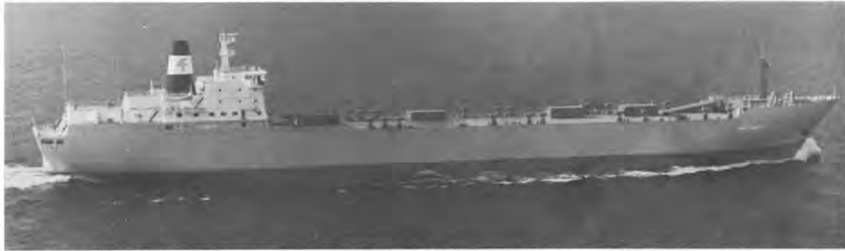
The 20,000-dwt MV Avon Forest, shown on trials, has a design speed of 19.5 knots when carrying automobiles.
