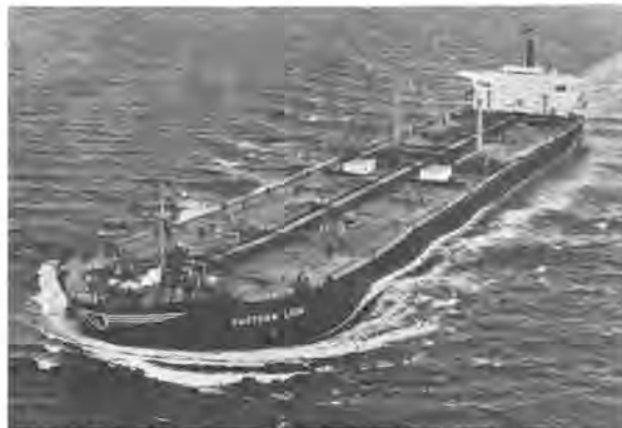
HITACHI DELIVERY: The Eastern Lion, a 264,914-dwt tanker built at Hitachi Zosen's Sakai shipyard, was recently delivered to her owner, Third United Shipping Corporation. Approximate dimensions of the tanker are: length between perpendiculars, 1,037 feet; molded breadth, 168 feet, and molded depth, 93 feet. Power is supplied by a Hitachi UA-320 type steam turbine developing a maximum output of 32,000 hp, providing a maximum trial speed of 16.1 knots.
