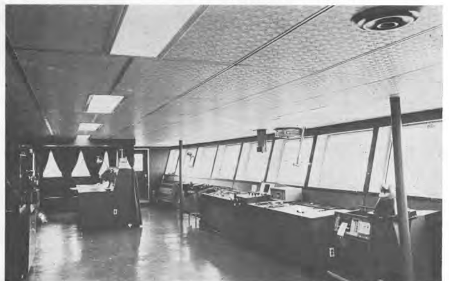
The unmanned machinery installation can be fully controlled from the bridge console shown in this view of the bridge. The bow thruster is controlled from the bridge wing.
