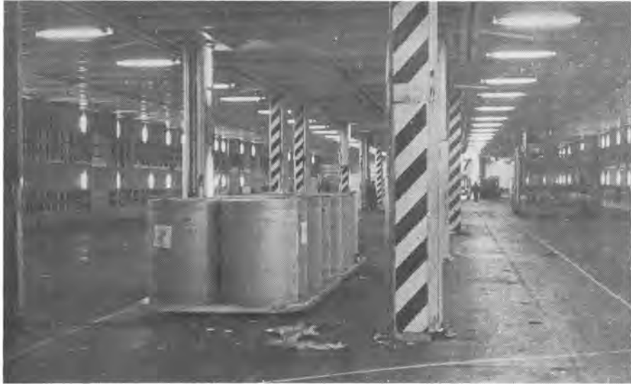
This view of the ro/ro deck shows a straddle carrier leaving after placing pallets with newsprint on an elevator for lowering to the decks below.
