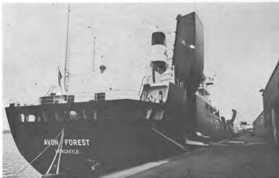
The Avon Forest unloading automobiles through special shell doors. These doors are located only on the starboard side—one forward and one aft. The ramp folds inboard.
