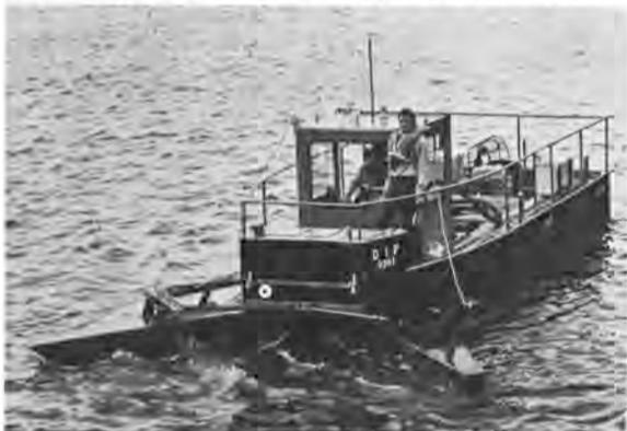
The DIP skimmers have the ability to harvest any floating material, including debris and sorbents, without changing the skimmer configuration.
