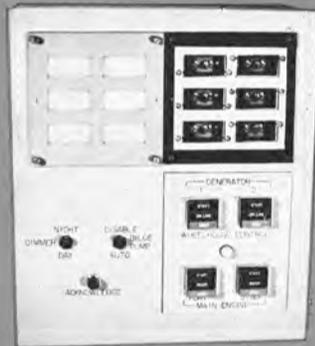
ENGINEER ROOM MONITOR UNIT Permits maximum utilization of engineroom manpower, provides indication of equipment status at any remote shipboard location, with control functions available on the bridge.
