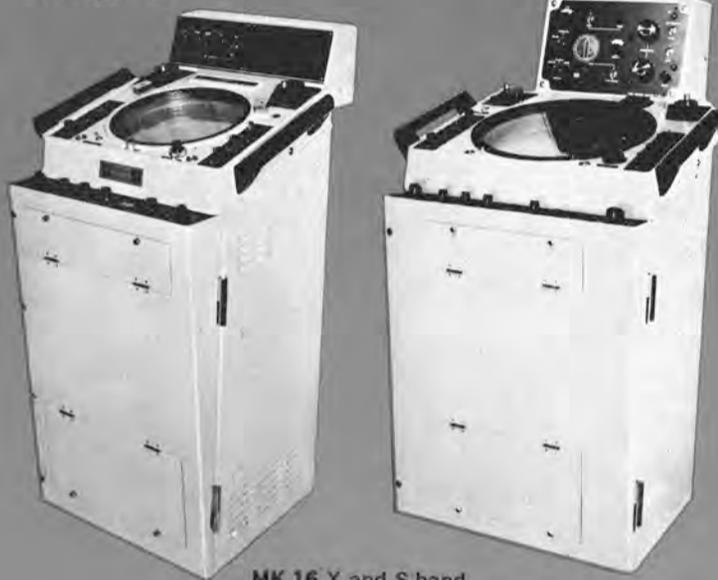
MK 16 X and S band heavy duty, 16-in. ppi, 30 and 50 kw peak power for top performance, accuracy and reliability. Full options.
