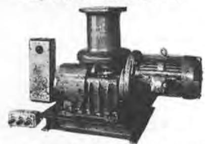
10 H.P.—220/440/3/60—1750 R.P.M.—Marine type reversing controller. Barrel diameter—10"—2 1/2" Flange. Height between flanges 12".
