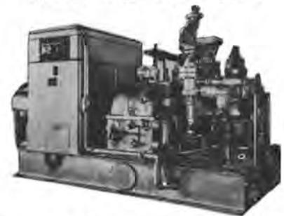
We offer with ABS or Lloyd's certificate. Our re-conditioning of this unit is fully guaranteed on a money-back basis. Has been through G.E. Engineering and the last stage has been rebladed with new style blading. All diaphragms re-machined.
