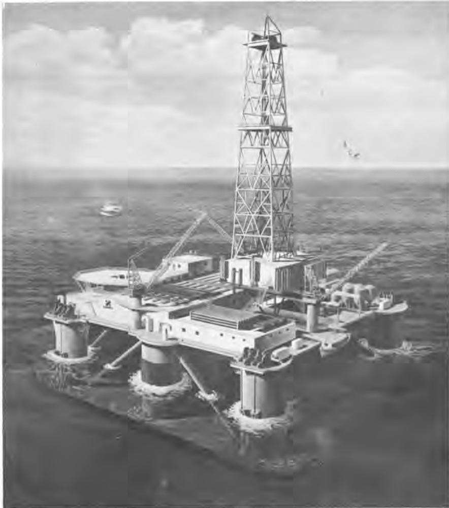
**ON THE COVER:** Three new U.S.-flag semisubmersible offshore drilling rigs like this artist's conception will be built for Zapata Off-Shore Company by Avondale Shipyards, Inc. in New Orleans. Construction on the advanced design, SS-2000 Class units will begin soon, with deliveries commencing in spring 1975.
