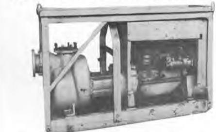
Reconditioned—mounted in portable steel frame. 1750 RPM—1100 GPM @ 100' head; 1500 GPM @ 70' head; 1800 GPM @ 50' head; 2100 GPM @ 20' head. Leroi gas engine—model D-201P3—4 x 4—1750 RPM—hand crank—wt. 600 lbs. **\$995**
