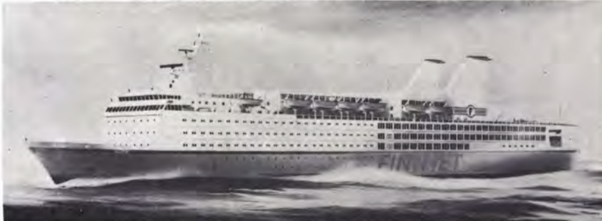
Artist's rendering of Finnjet, a planned new, high-speed Finnish passenger liner, shows twin exhaust stacks for the ship's two Pratt & Whitney Aircraft FT4 marine gas turbines sold by Turbo Power & Marine Systems of Farmington, Conn., a subsidiary of United Aircraft Corporation.
