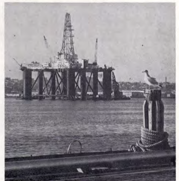
FROM HALIFAX: Ready for oil exploration in the North Sea, this Halifax-built semisubmersible, Sedneth 701, is shown undergoing tests for its thrusters in Halifax Harbor. The unit is one of six semisubmersibles for the oil industry, either built by or on order with the Halifax Shipyards. Sedneth 701 will be delivered to its owners, Nederlandse Zeebormaatshappij B.V. (Sea Drilling Netherlands).
