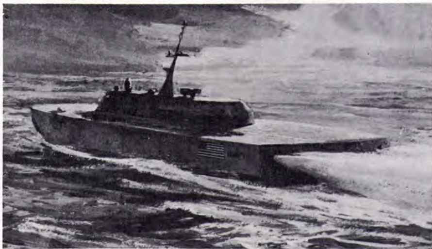
An artist's conception of the Navy's surface effect ship which will be capable of operating in open seas at speeds in excess of 80 knots.
