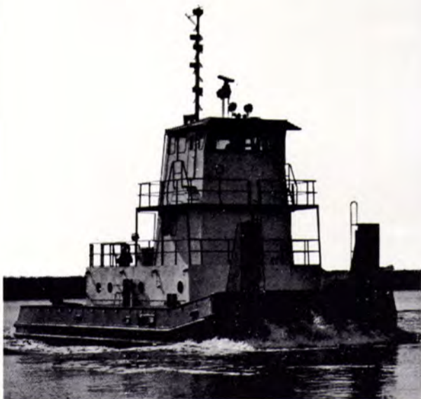
E. N. Belcher, Jr. Fort Myers, Florida 70 x 27 x 9.5 Twin D-379 Caterpillar, 1100 HP
