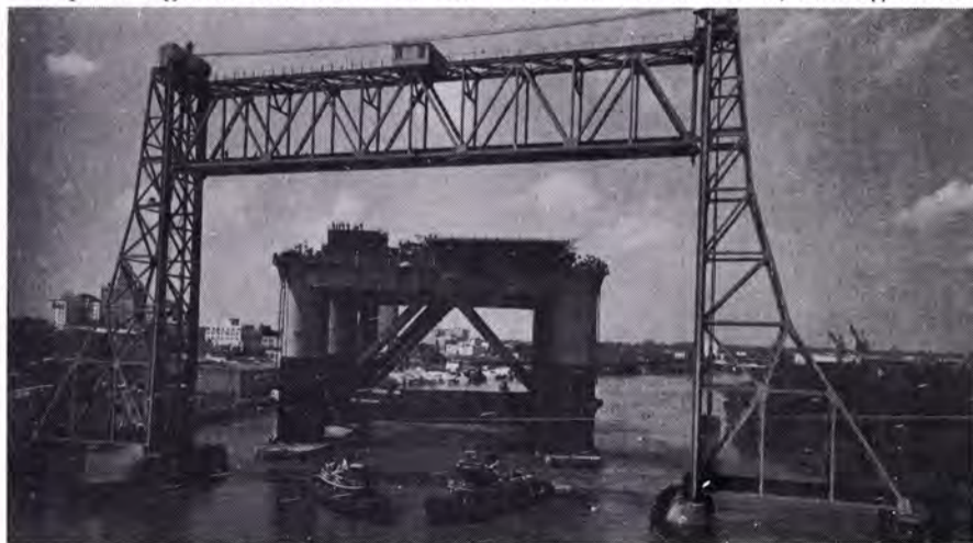
The Zapata Uglund is shown as she was moved from Bethlehem Shipyard, Beaumont, Texas, to her completion site. The giant semisubmersible rig cleared this railroad drawbridge with just a few feet to spare.
