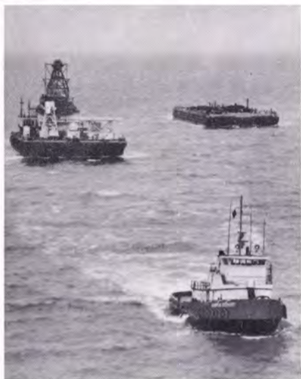
ALL-OCEAN TUG, MISTER RICHARD , equipped with two ALCO, V-12, 251s rated at 2650 BHP each has 13 knots free-running speed.
