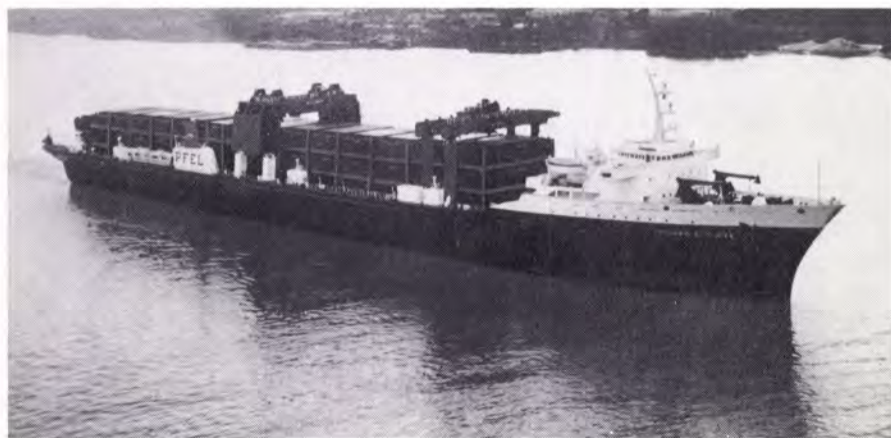
LASH VESSEL, THOMAS E. CUFFE's ship service is provided by ALCO 16-cylinder diesel rated at 2,000 KW at 900 RPM.
