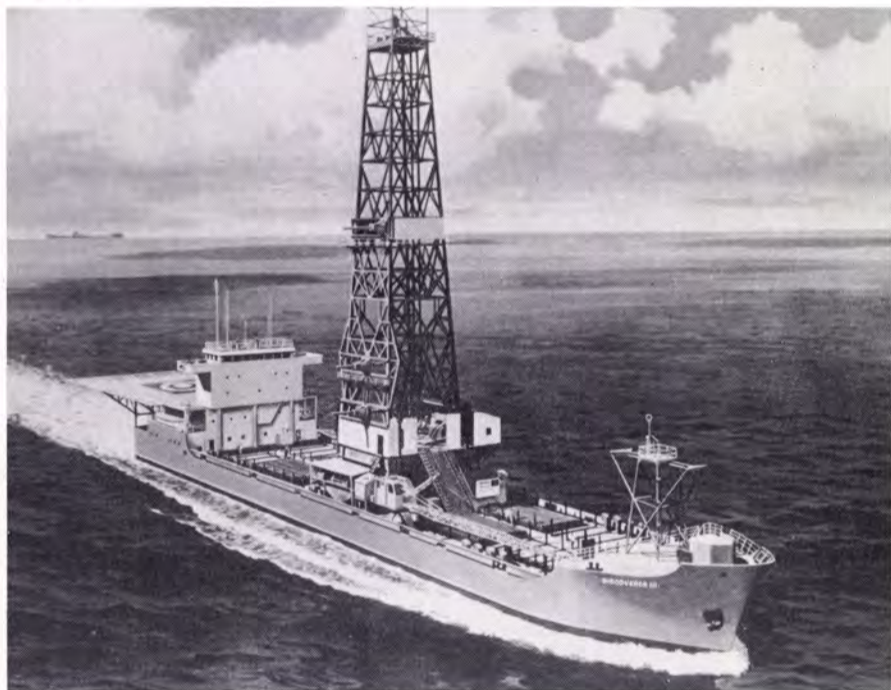
DRILL SHIP DISCOVERER III obtains main propulsion from three, 12-cylinder, ALCO 251s.
