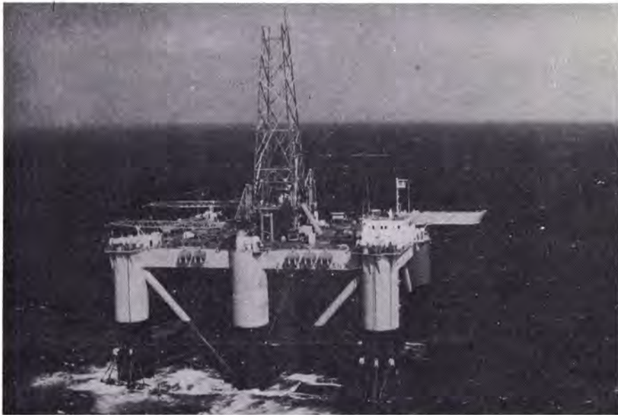
The giant rig registered speeds of up to 11 knots during its sea trials in the Gulf of Mexico. The vessel is shown in partially ballasted position, with her derrick incomplete.
