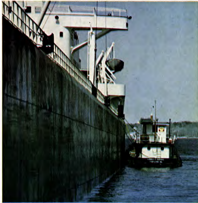
Golten Ship Repair tank boat, the Aubrey L. Hudgins, pumps Shell MELINA Oil into ship in mid-harbor at Portland, Maine. The Hudgins' pumps can deliver 4,800 gallons per hour from her 48,000-gallon-capacity tanks. Turnaround time for ships is speeded up by this fast, clean delivery system.
