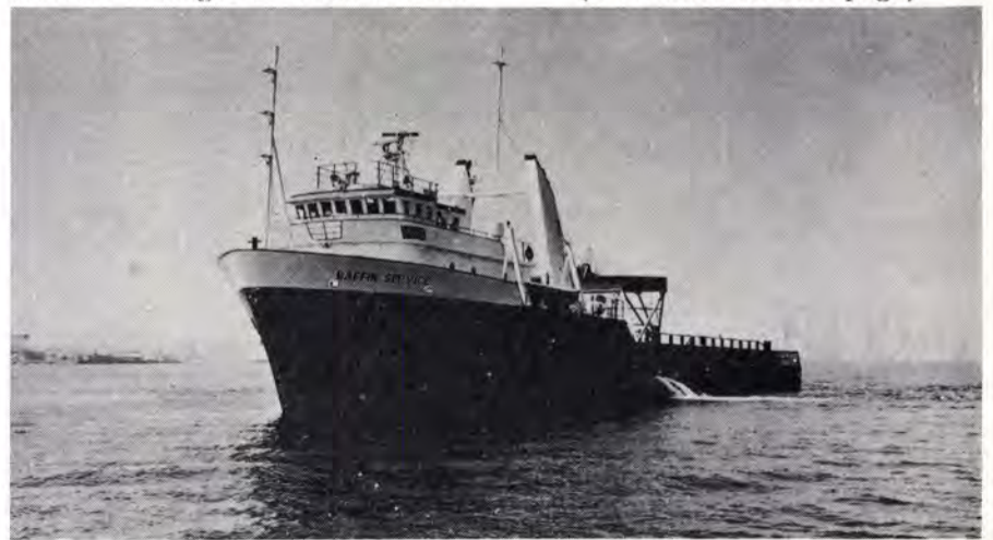
The 6,560-horsepower rugged tug/supply/anchor handling vessel Baffin Service will accompany the new semisubmersible Zapata Uglund to her initial assignment in the North Sea.
