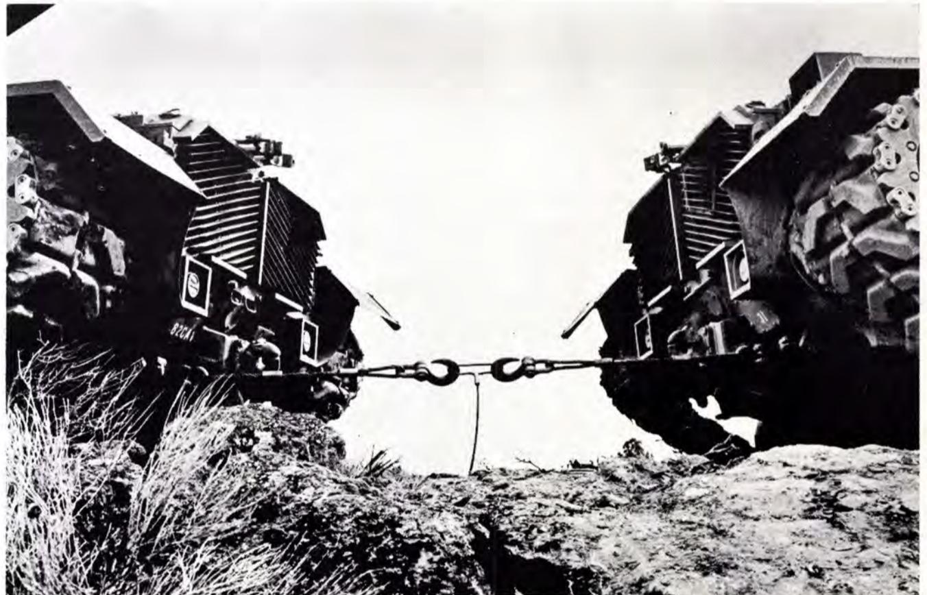
We put three different swaged sleeves through the toughest torture test we could devise: a side-pull test designed to tear wire rope slings apart at the sleeves. This is what happened: In a tug of war between two 52-ton tanks, the 1/2" aluminum and carbon sleeves ripped apart, but the ESCO 1/2" stainless duplex sleeve wouldn't give up.
