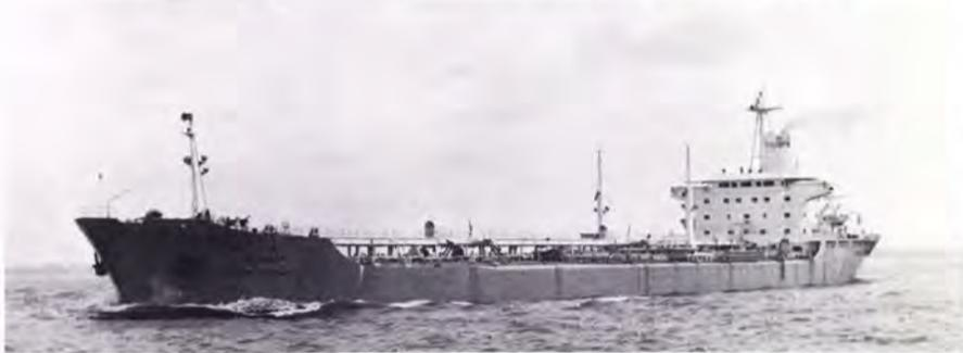
The Marsa El Hariga, powered by an AESA/Sulzer main engine, has a cargo capacity of approximately 1,984,171 cubic feet.
