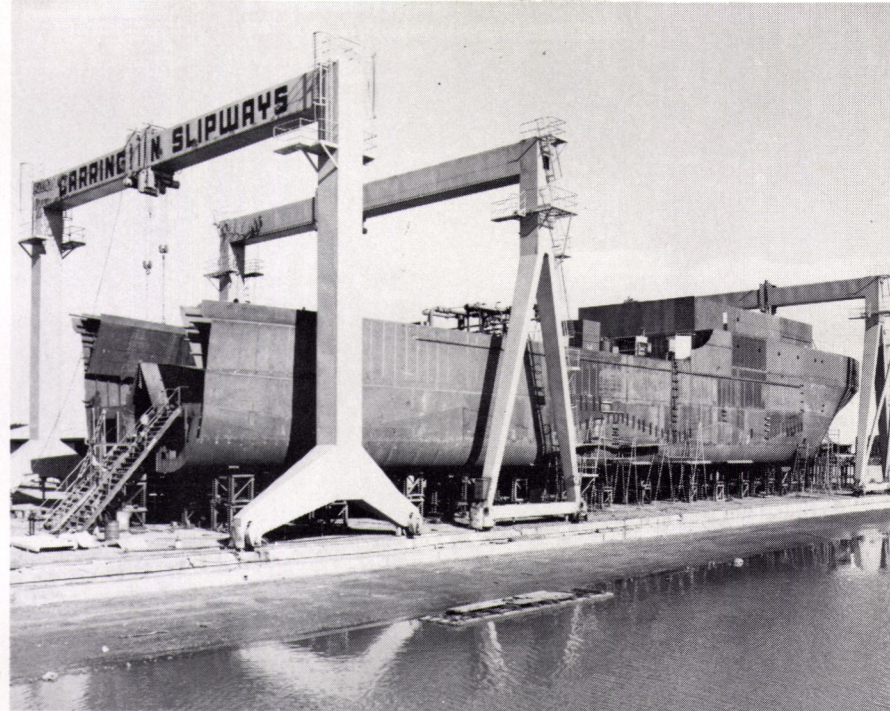
The 4,000-ton cement carrier being built by Carrington Slipways of Tomago, Australia, for Bulkships Container Ltd. is shown 163 working days after signing of design and building contract.
