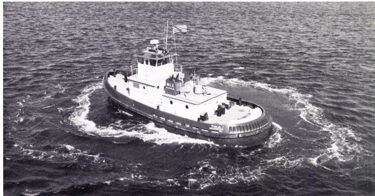
The twin-screw 360-degree rotating Kort nozzle shipdocking tug Tina is powered by two General Motors Detroit Diesel engines generating 1,070 horsepower.
