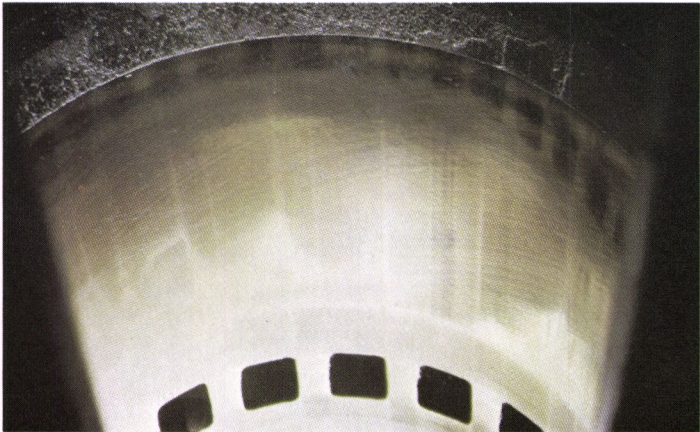
After 18,864 hours this cylinder liner from an EMD-12 645 E5 still shows original crosshatch marks. A tribute to the excellent wear protection of Shell Tornus Oil.
