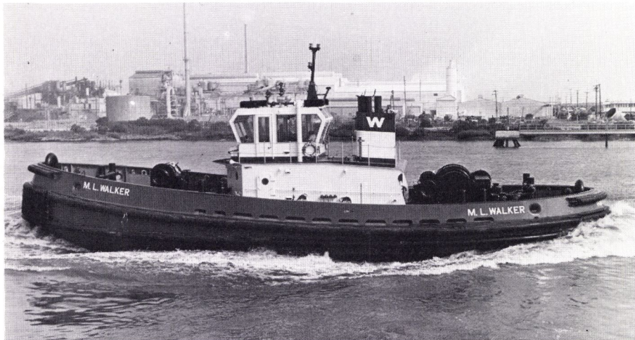
The M.L. Walker, shown above during trials, and her sistership H. Burgess require space only the length of their hulls (96 feet) to make a complete turn.
