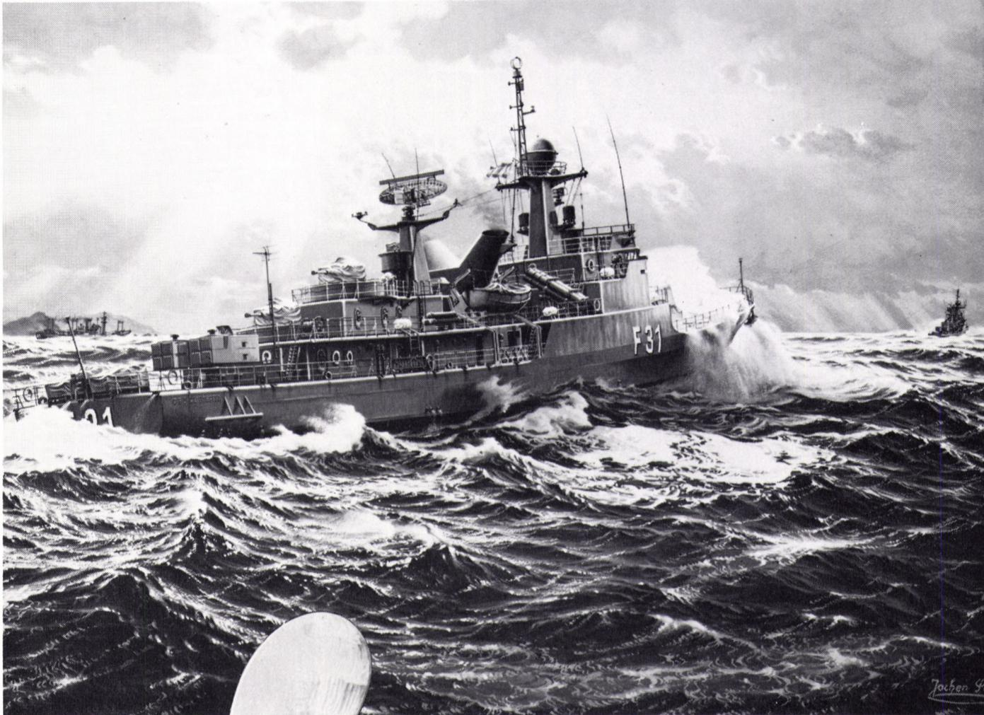
Corvette "DESCUBIERTA" and 7 sister ships with two Escher Wyss controllable pitch propellers
