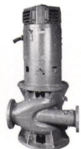
Gardner-Denver — bronze — vertical — total suction lift 15' — 8" suction — 6" discharge — 1500 GPM @ 25 lbs — 1750 RPM. MOTOR: 30 HP — 230 VDC — 112 amps — made by Century.
