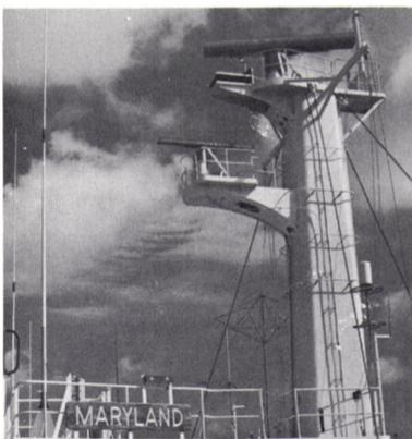
Mast with ATLAS S-Band & X-Band Antennas
