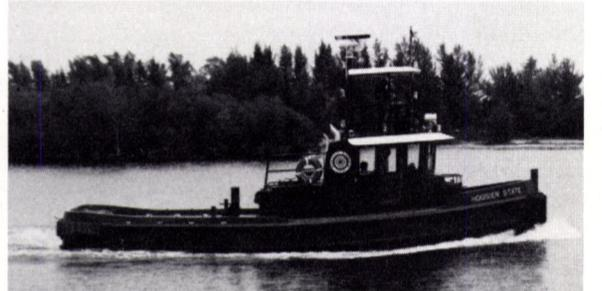
The Petchul-designed Hoosier State provides control both from the pilothouse and a fly-bridge station located on top of the pilothouse.
